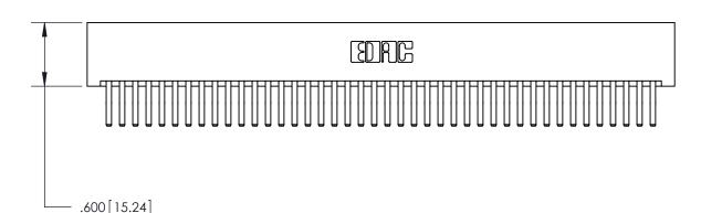
Card Slot Accepts .054 [1.37] to .070 [1.78] Thick P.C. Board .330 [8.38] Card Slot .160 [4.07] Point of Contact -
