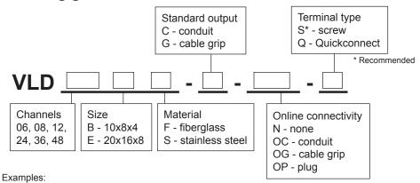
VLD06BF-C-OG-S: 6 channel switchbox, fiberglass 10x8x4 enclosure with screw terminals and conduit outputs, online connectivity with cable grip output
