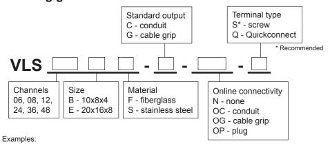
VLS06BF-C-OG-S: 6 channel switchbox, fiberglass 10x8x4 enclosure with screw terminals and conduit outputs, online connectivity with cable grip output
