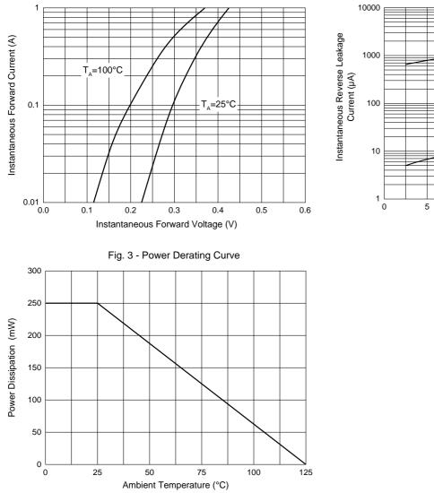
Fig. 1 - Typical Instantaneous Forward Characteristics
