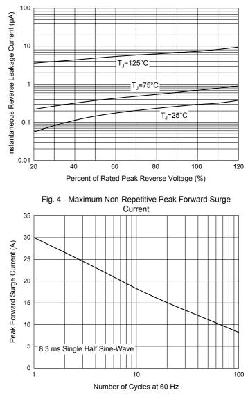
Fig. 2 - Typical Reverse Leakage Characteristics
