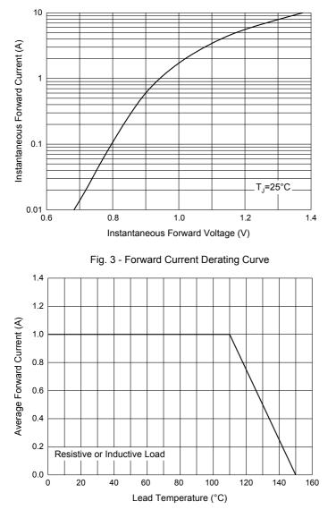
Fig. 1 - Typical Instantaneous Forward Characteristics
