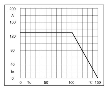
**Fig5.Forward Current Derating Curve**
