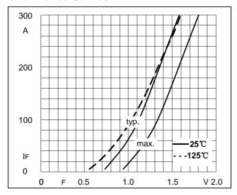
Fig1. Forward Characteristics
