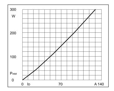
Fig2. Power dissipation
