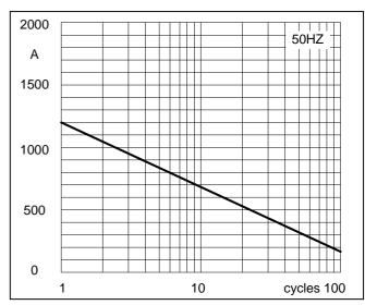
Fig4. Max Non-Repetitive Forward Surge Current
