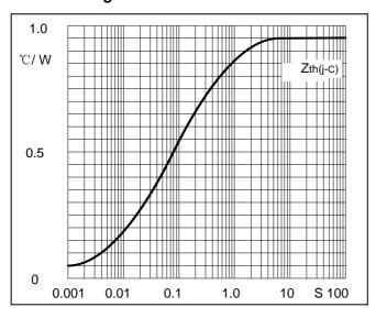
Fig3. Transient thermal impedance
