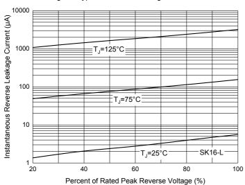
Fig. 8 - Typical Reverse Leakage Characteristics
