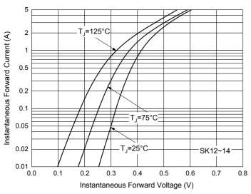
Fig. 5 - Typical Instantaneous Forward Characteristics
