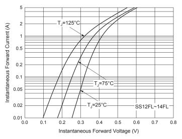
Fig. 5 - Typical Instantaneous Forward Characteristics
