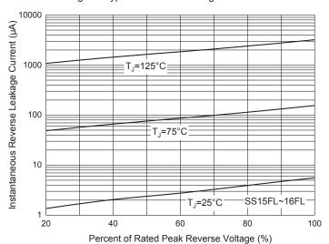
Fig. 8 - Typical Reverse Leakage Characteristics
