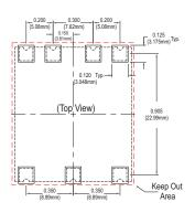
\* Do not route any traces in the keep out area. It is recommended the next layer under the keep out area is to be ground plane.
