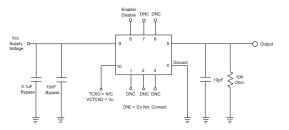
TV Series Clipped Sinewave Test Circuit
