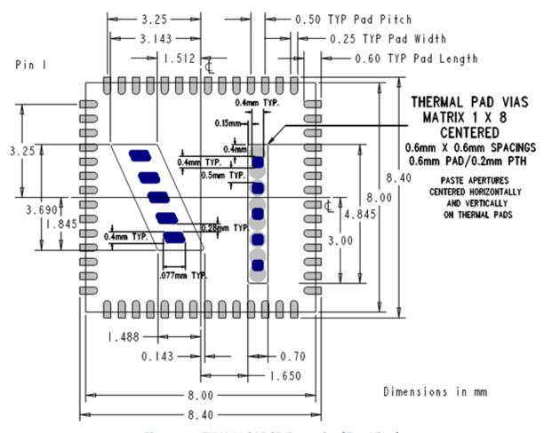
Figure 14: EN6382QI PCB Footprint (Top View)
