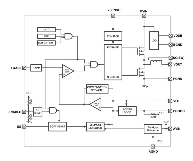
Figure 4: Functional Block Diagram
