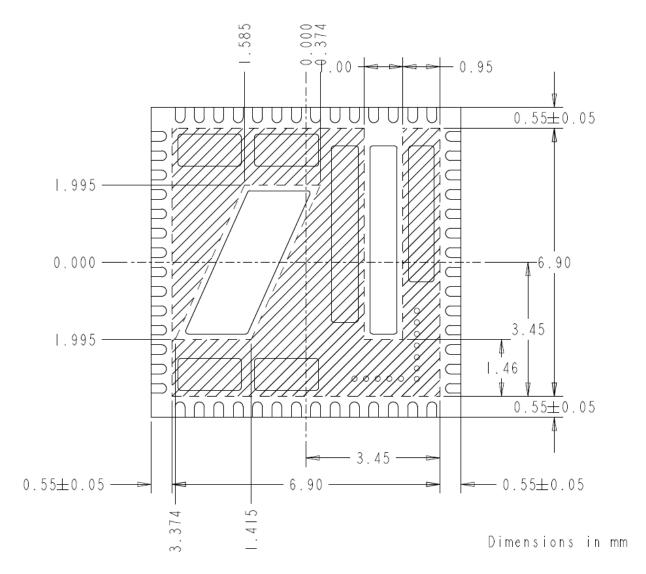
Figure 13: EN6382QI Package - PCB Footprint Keepout (Bottom view)
