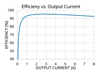
Figure 2: Efficiency at VIN = 5V, VOUT = 3.3V
