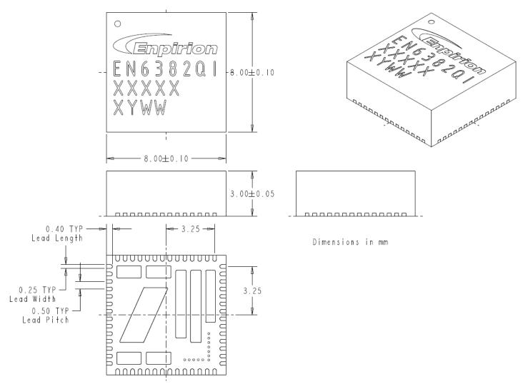
Figure 15: EN6382QI Package Dimensions
