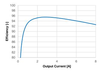
Figure 6: Efficiency V<sub>IN</sub> =5.5V, V<sub>OUT</sub> = 3.3V
