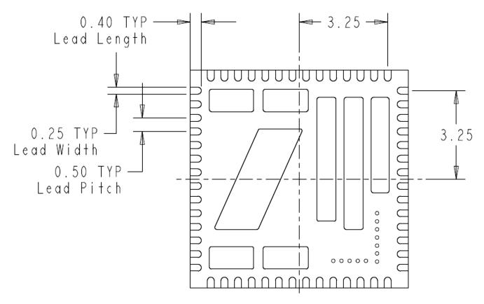
Figure 12: Lead-Frame exposed metal (Bottom View)
