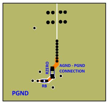
Figure 10: Inner Layer 3 - routing
