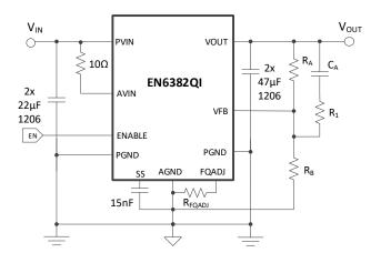
**Figure 1: Simplified Applications Circuit**
