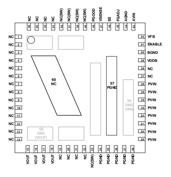
Figure 3: Pin Diagram (Top View)
