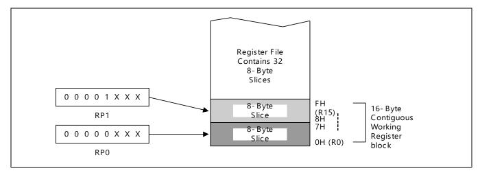
Figure 2-7 Contiguous 16 Byte Working Register Block
