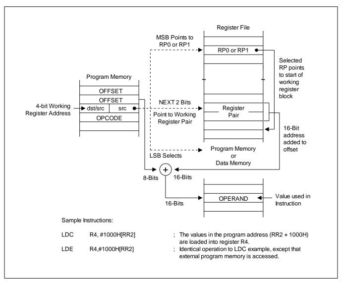
*Figure 3-9* illustrates the indexed addressing to program or data memory.
