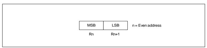
Figure 2-9 16-Bit Register Pair
