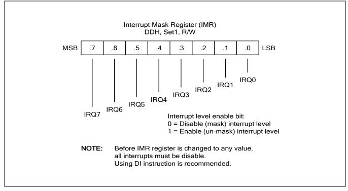
Figure 5-6 illustrates the interrupt mask register (IMR).
