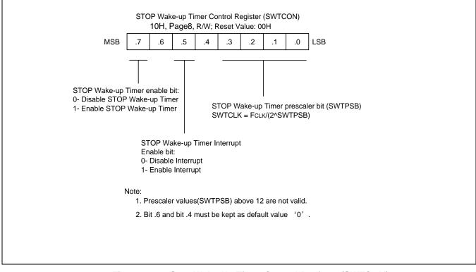
Figure 12-1 Stop Wake-Up Timer Control Register (SWTCON)
