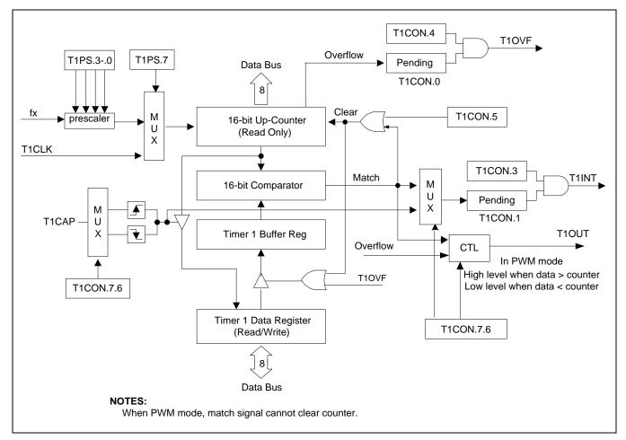
Figure 13-6 illustrates the functional block diagram of Timer 1.
