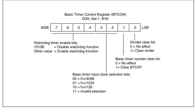
Figure 10-1 Basic Timer Control Register (BTCON)
