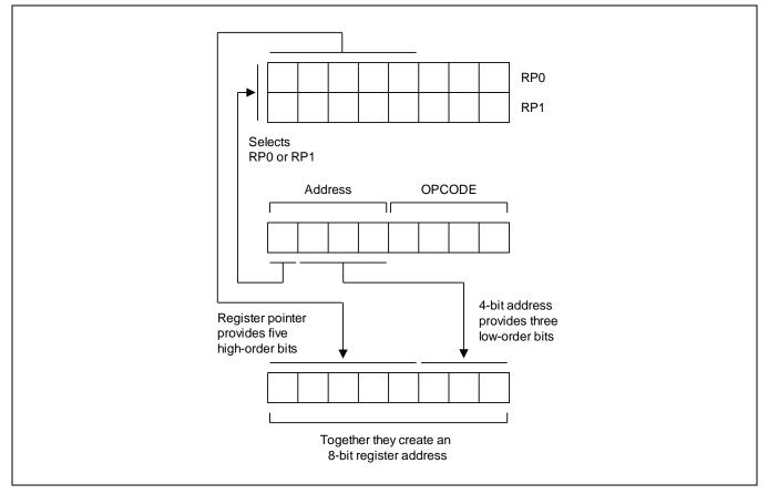
*Figure 2-12* illustrates the 4-bit working register addressing.
