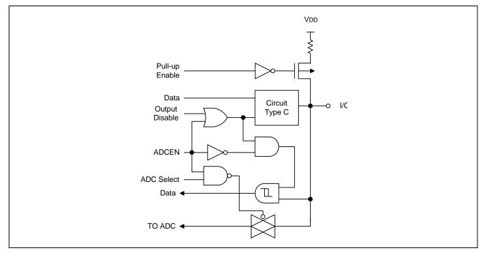
Figure 1-6 Pin Circuit Type F-16 (P0)
