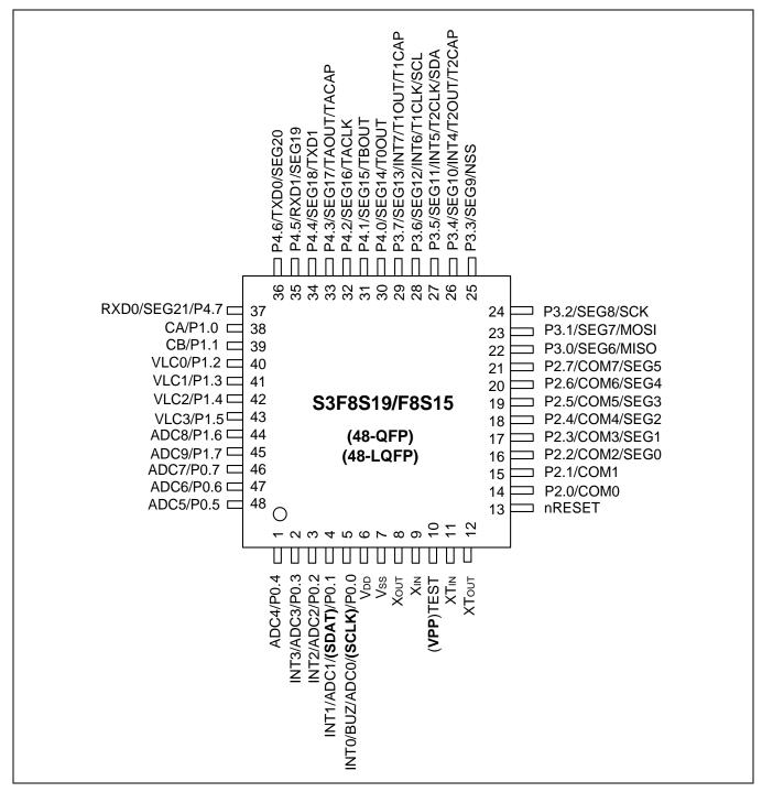
Figure 25-1 S3F8S19/S3F8S15 Pin Assignments
