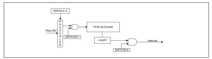
Figure 12-2 Stop Wake-Up Timer Functional Block Diagram
