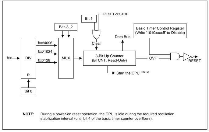
Figure 10-2 Basic Timer Block Diagram
