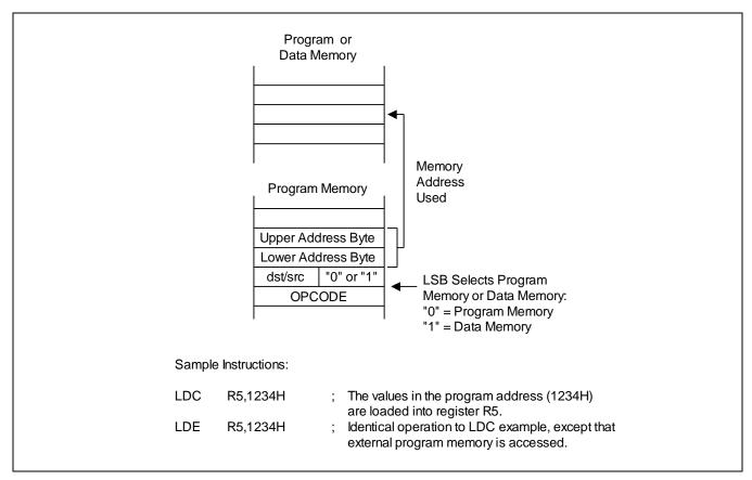
Figure 3-10 Direct Addressing for Load Instructions
