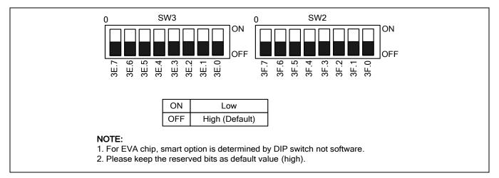
Figure 26-3 DIP Switch for Smart Option
