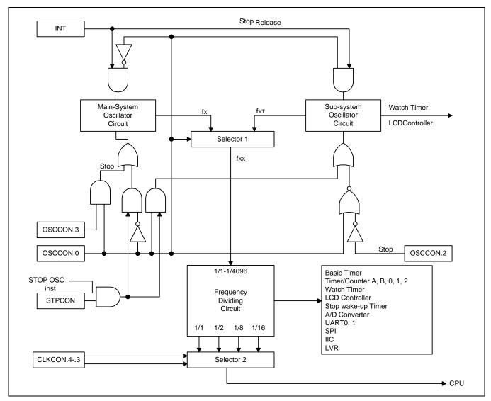
Figure 7-10 System Clock Circuit Diagram
