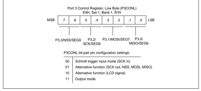
Figure 9-9 Port 3 Low-Byte Control Register (P3CONL)
