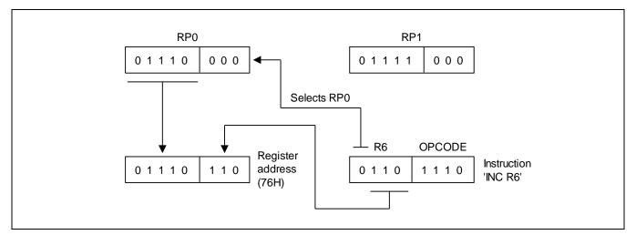
Figure 2-13 4-Bit Working Register Addressing Example
