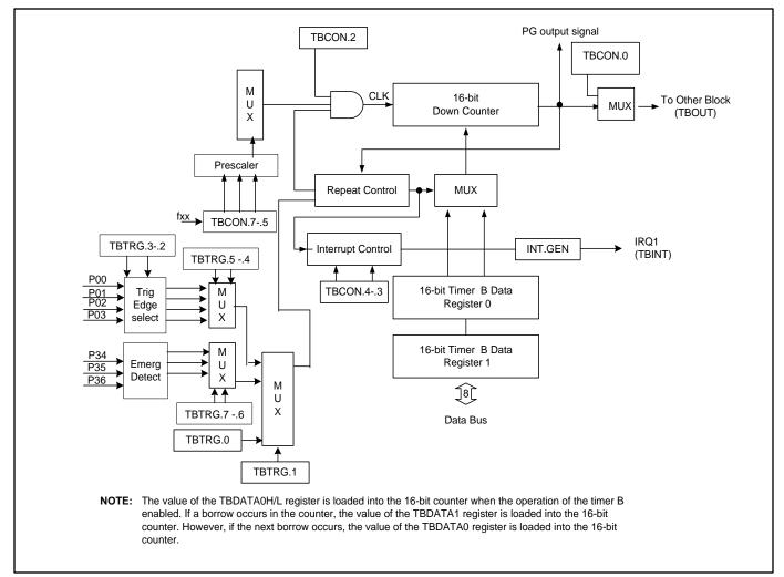
Figure 13-14 Timer B Functional Block Diagram
