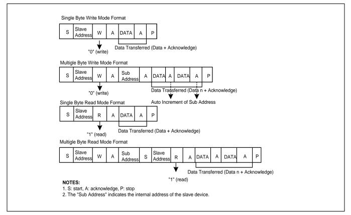
Figure 18-9 I2C Bus Interface Data Formats
