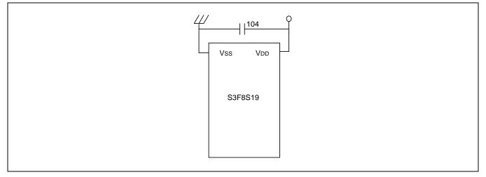
Figure 23-6 The Circuit Diagram to Improve EFT Characteristics
