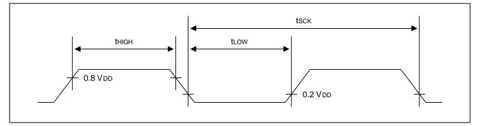
Figure 23-4 Waveform for UART Timing Characteristics
