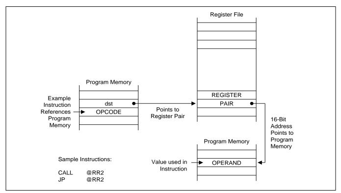
Figure 3-4 Indirect Register Addressing to Program Memory
