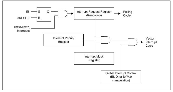
Figure 5-4 Interrupt Function Diagram
