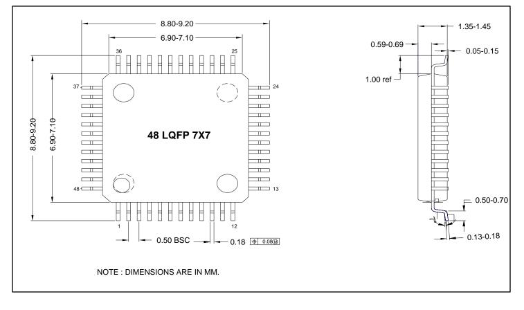
Figure 24-2 48-LQFP Package Dimensions
