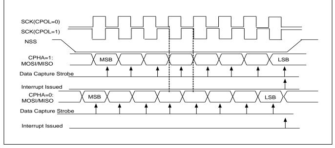
Figure 17-2 SPI Data Timing
