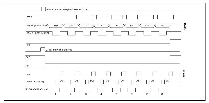
Figure 20-6 Timing Diagram for Serial Port Mode 0 Operation
