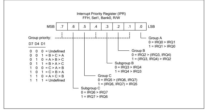
Figure 5-8 Interrupt Priority Register (IPR)
