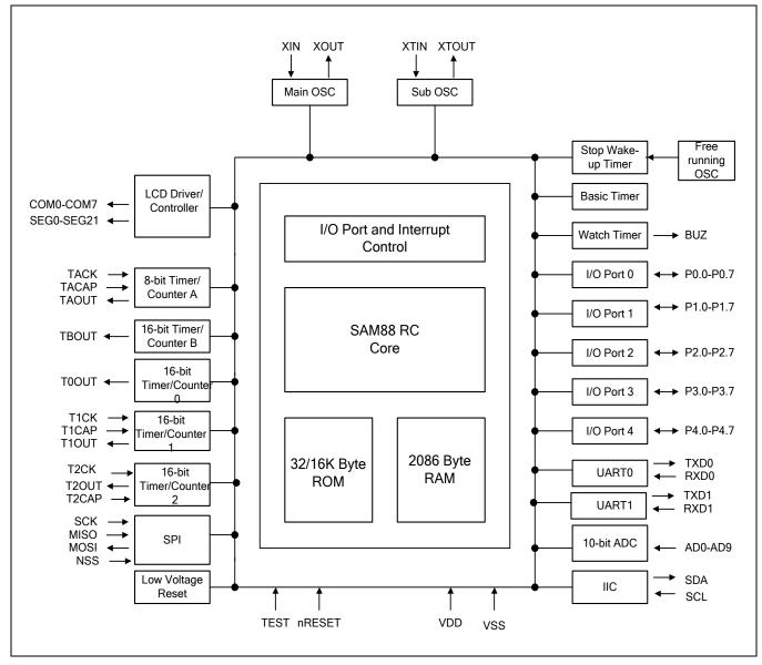
Figure 1-1 S3F8S19/S3F8S15 Block Diagram
