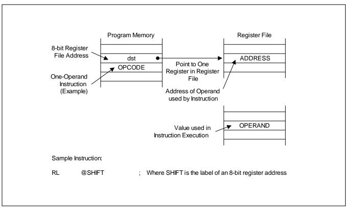
Figure 3-3 illustrates the indirect register addressing to register file.
