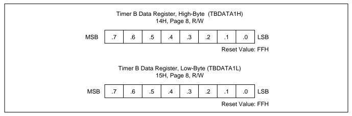
Figure 13-13 Timer B Data Registers (TBDATA1H/L)
