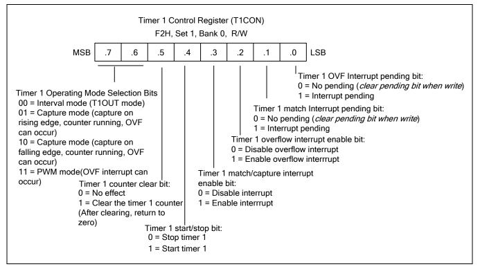
Figure 13-4 Timer 1 Control Register (T1CON)
