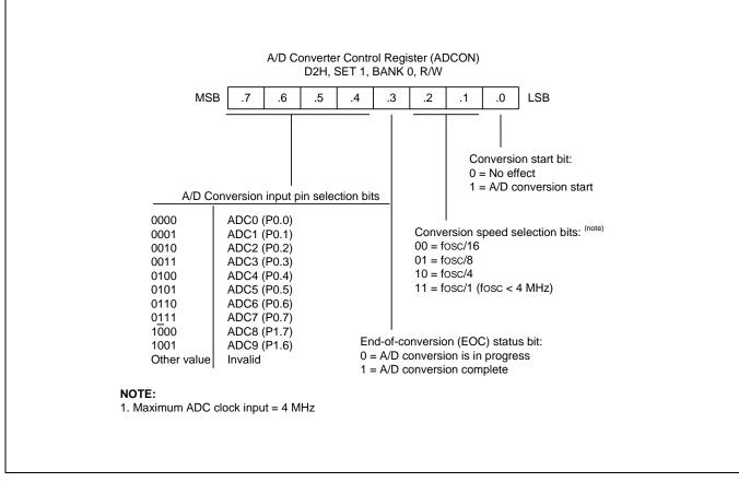
*Figure 16-1* illustrates the A/D converter control register (ADCON).
