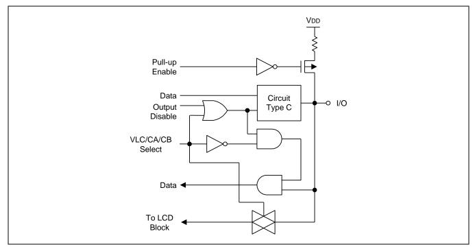
Figure 1-9 Pin Circuit Type F-17(P1)
