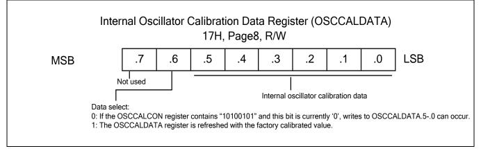
Figure 7-6 Internal Oscillator Calibration Data Register (OSCCALDATA)
