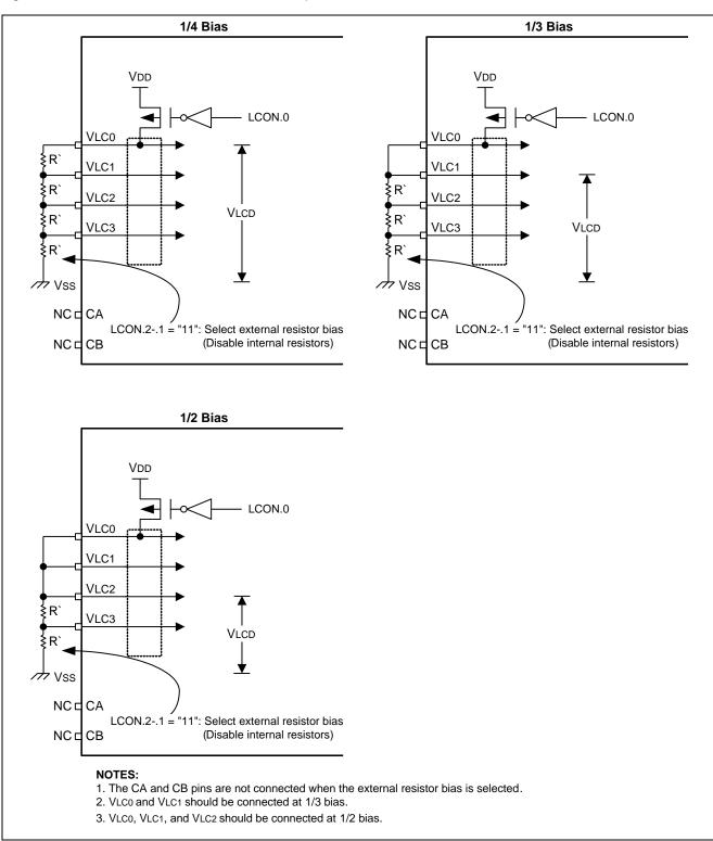
*Figure 15-7* illustrates the external resistor bias pin connection.
