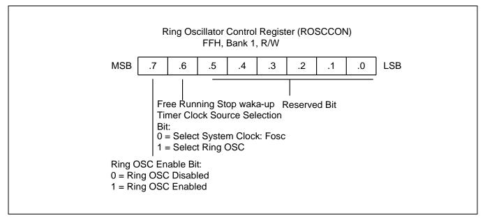
Figure 7-8 Ring Oscillator Control Register (ROSCCON)
