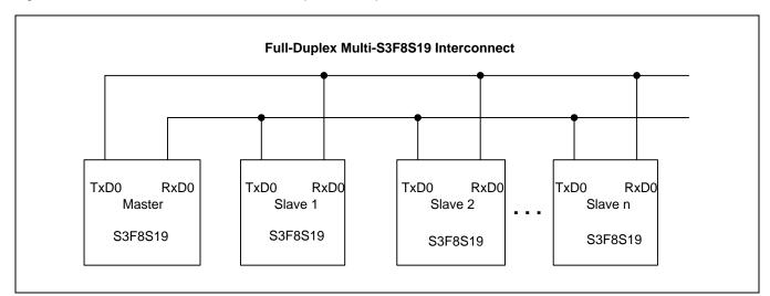
Figure 19-10 illustrates the connection example of multiprocessor serial data communications.
