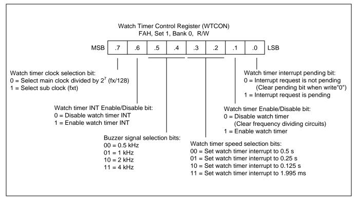
Figure 14-1 Watch Timer Control Register (WTCON)
