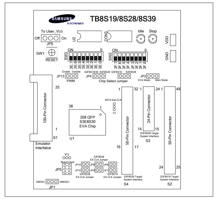
Figure 26-2 TB8S19/8S28/8S39 Target Board Configuration
