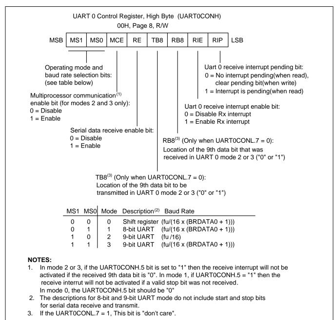
*Figure 19-1* illustrates the UART 0 high byte control register.
