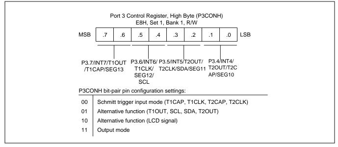
Figure 9-8 Port 3 High-Byte Control Register (P3CONH)
