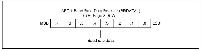
Figure 20-4 UART 1 Baud Rate Data Register (BRDATA1)
