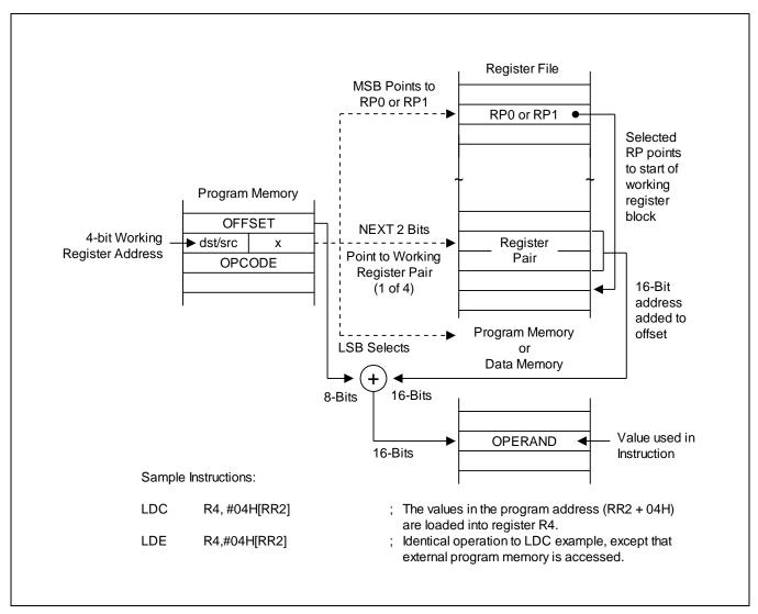
Figure 3-8 illustrates the indexed addressing to program or data memory with short offset.
