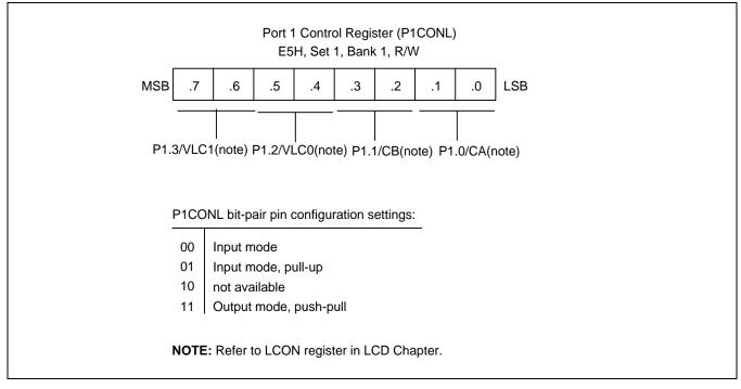
Figure 9-5 Port 1 Control Register Low Byte
