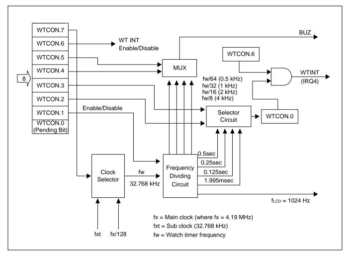
Figure 14-2 Watch Timer Circuit Diagram
