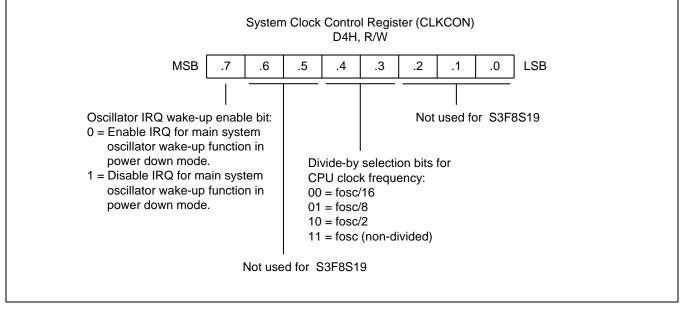
Figure 7-4 System Clock Control Register (CLKCON)
