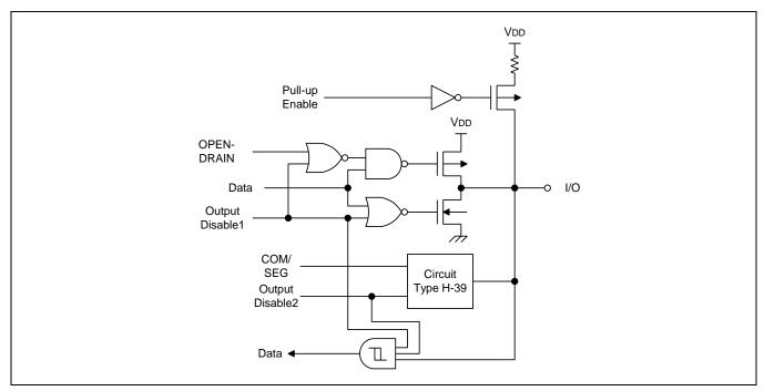
Figure 1-10 Pin Circuit Type H-41 (P3)
