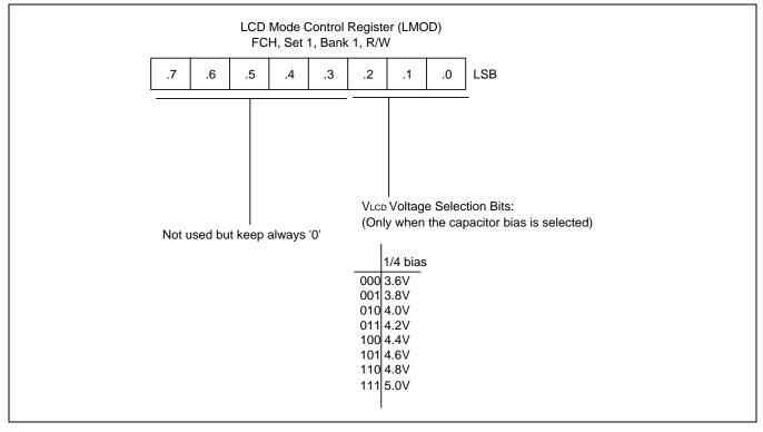
Figure 15-5 LCD Mode Control Register (LMOD)
