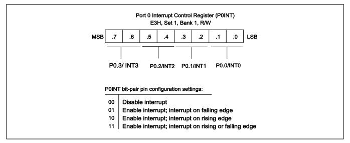
Figure 9-3 Port 0 Interrupt Control Register (P0INT)
