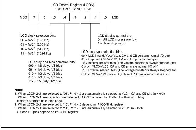
Figure 15-4 LCD Control Register (LCON)
