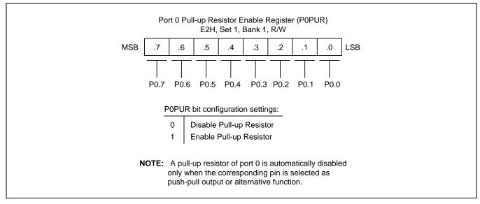
Figure 9-2 Pull-Up Resistor Enable Register (P0PUR)
