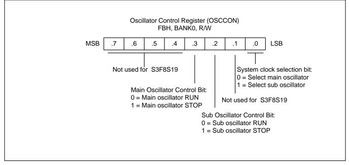
Figure 7-7 Oscillator Control Register (OSCCON)
