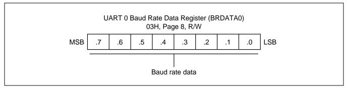
Figure 19-4 UART 0 Baud Rate Data Register (BRDATA0)
