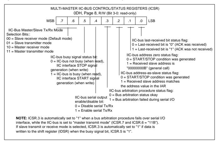
Figure 18-2 Multi-Master I2C Bus Control/Status Register (ICSR)
