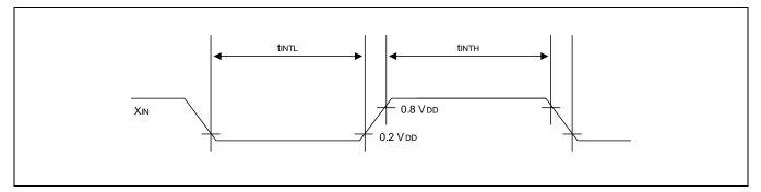
Figure 23-1 Input Timing Measurement Points
