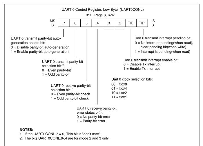
Figure 19-2 illustrates the UART 0 low byte control register.
