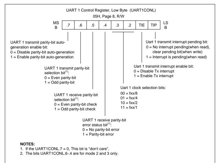
Figure 20-2 illustrates the UART 1 low byte control register.
