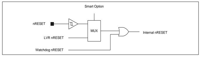
Figure 8-2 Reset Block Diagram
