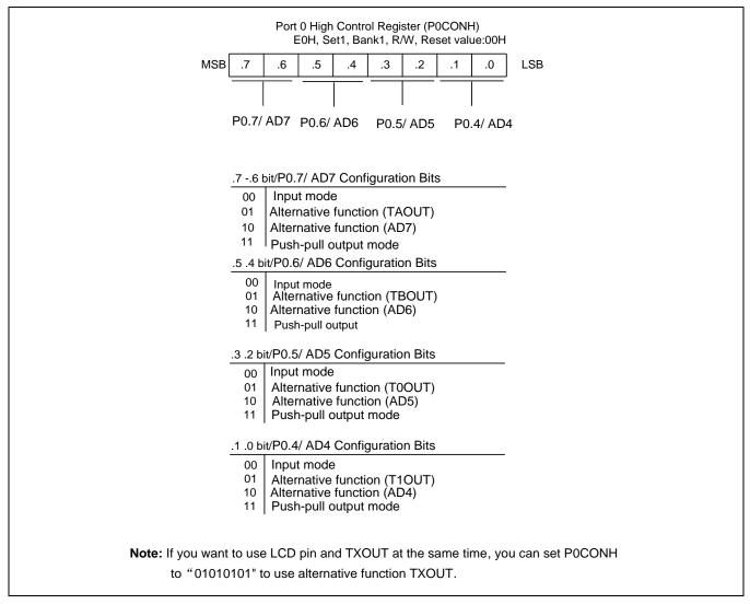
Figure 9-1 Port 0 Control Register High Byte (P0CONH)
