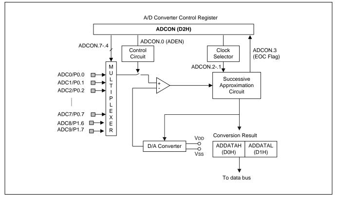
Figure 16-2 A/D Converter Circuit Diagram
