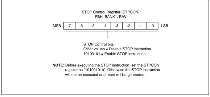
Figure 7-9 STOP Control Register (STPCON)
