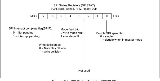
Figure 17-4 SPI Status Register (SPISTAT)
