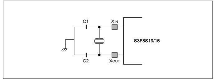
Figure 7-2 Main Oscillator Circuit (Crystal/Ceramic Oscillator)
