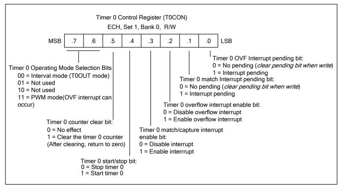
Figure 13-1 Timer 0 Control Register (T0CON)
