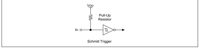
Figure 1-4 Pin Circuit Type B
