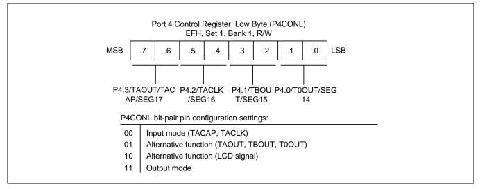
Figure 9-15 Port 4 Low-Byte Control Register (P4CONL)
