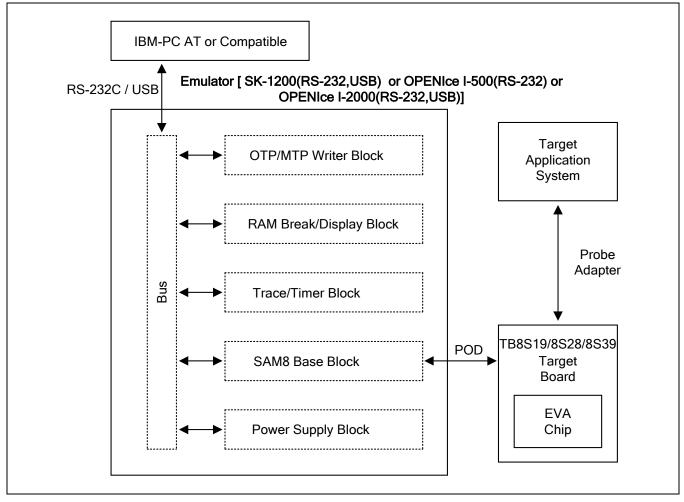
Figure 26-1 Development System Configuration
