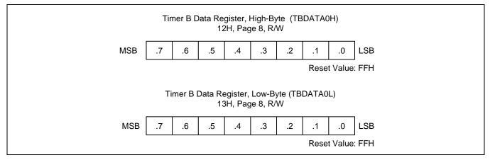
Figure 13-12 Timer B Data Registers (TBDATA0H/L)
