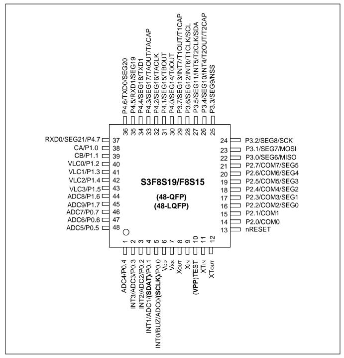
Figure 1-2 S3F8S19/S3F8S15 Pin Assignments (48-QFP and 48-LQFP)
