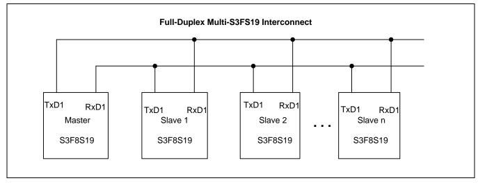
*Figure 20-10* illustrates the connection example of multiprocessor serial data communications
