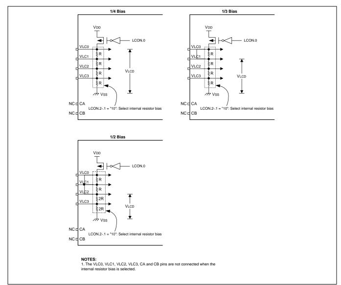
*Figure 15-6* illustrates the internal resistor bias pin connection.
