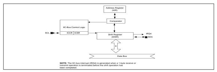
Figure 18-4 illustrates the multi-master I2C bus address register.
