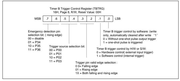
Figure 13-11 Timer B Trigger Register (TBTRG)
