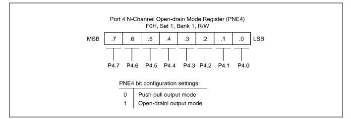
Figure 9-17 Port 4 N-Channel Open-Drain Mode Register (PNE4)
