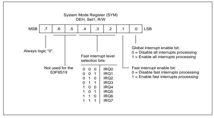
Figure 5-5 illustrates the system mode register (SYM).
