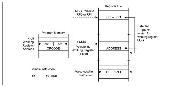
Figure 3-5 Indirect Working Register Addressing to Register File
