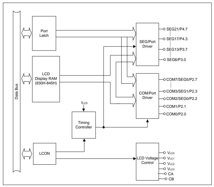
Figure 15-2 LCD Circuit Diagram
