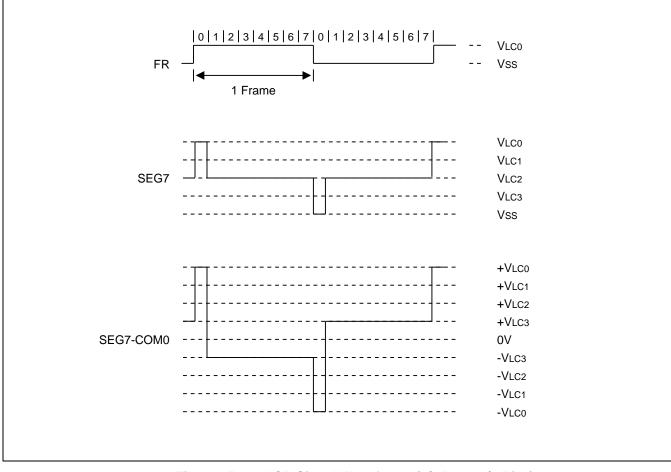
Figure 15-14 LCD Signal Waveforms (1/8 Duty, 1/4 Bias)
