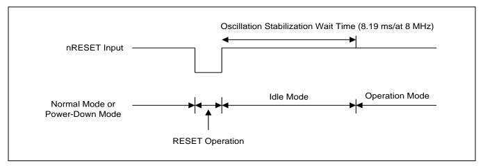
Figure 8-3 Timing for S3F8S19/S3F8S15 After RESET
