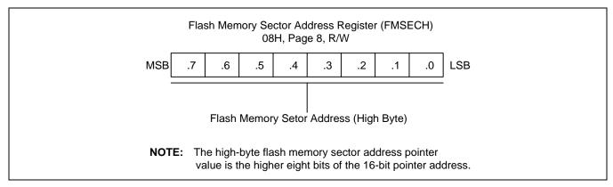
Figure 21-3 illustrates the Flash memory sector address register high byte.
