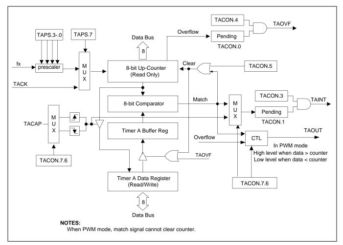
Figure 11-3 illustrates the timer A functional block diagram.
