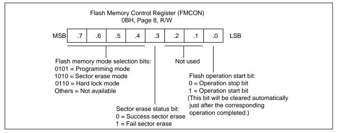
Figure 21-1 Flash Memory Control Register (FMCON)
