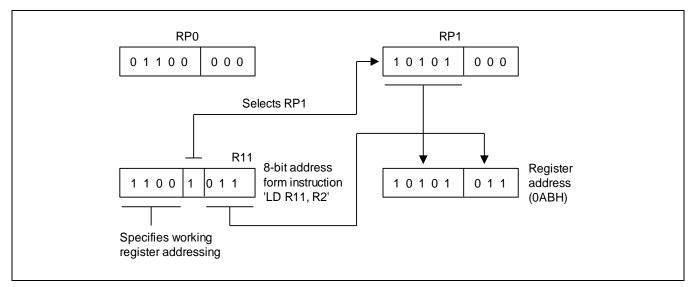
Figure 2-15 8-Bit Working Register Addressing Example
