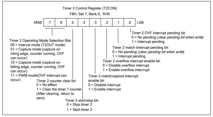
Figure 13-7 Timer 2 Control Register (T2CON)
