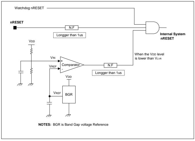
Figure 22-1 Low Voltage Reset Circuit
