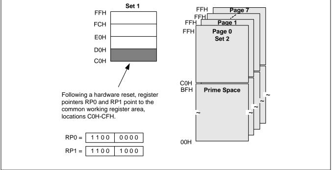
Figure 2-11 Common Working Register Area
