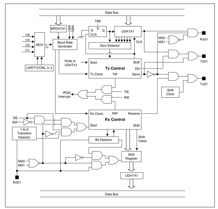
Figure 20-5 illustrates the functional block diagram of UART 1.
