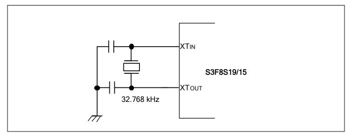
Figure 7-3 Sub-System Oscillator Circuit (Crystal Oscillator)
