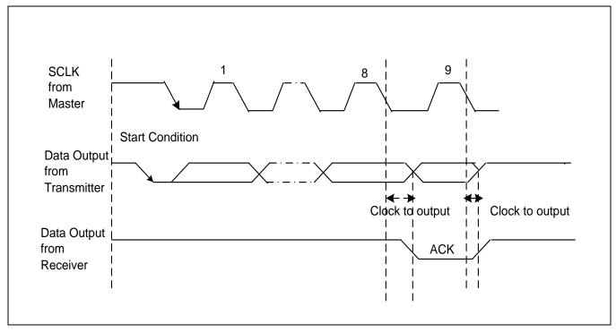
Figure 18-10 Acknowledge Response from Receiver
