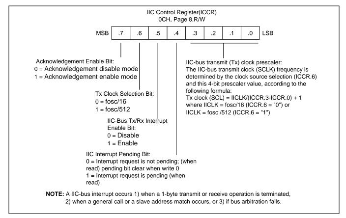
Figure 18-1 illustrates the multi-master I2C bus control register.
