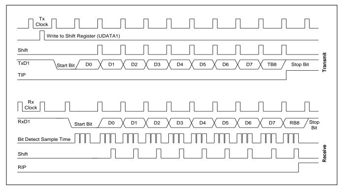
Figure 20-9 Timing Diagram for Serial Port Mode 3 Operation
