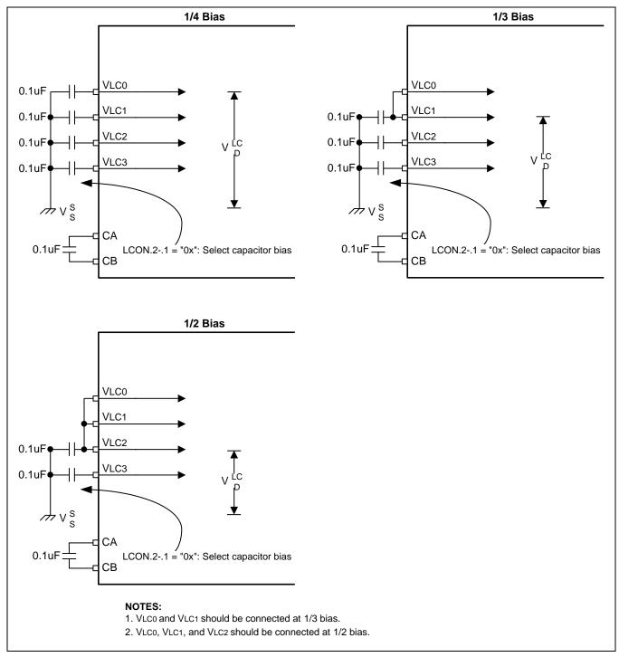
Figure 15-8 Capacitor Bias Pin Connection
