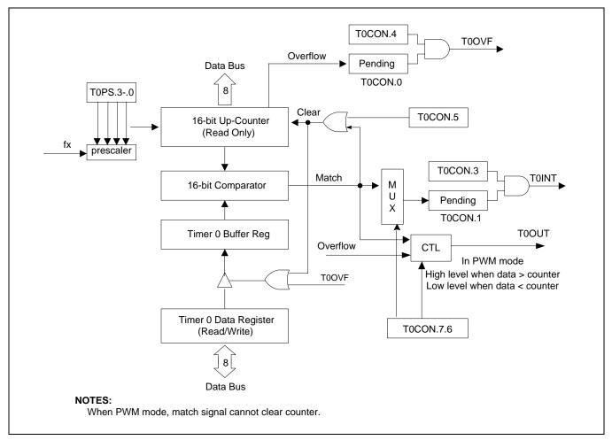
Figure 13-3 Timer 0 Functional Block Diagram
