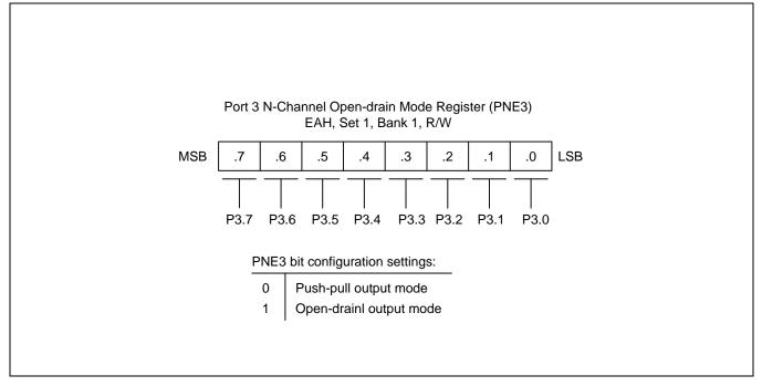
Figure 9-13 Port 3 N-Channel Open-Drain Mode Register (PNE3)
