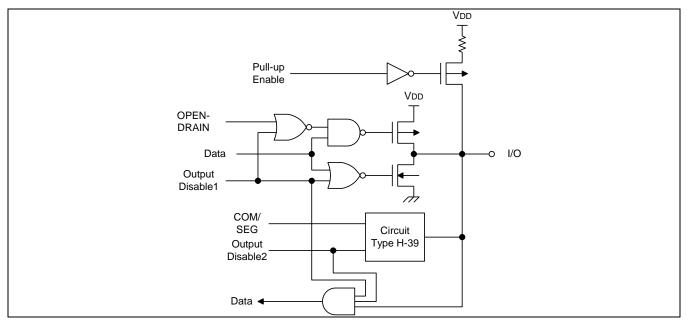
Figure 1-11 Pin Circuit Type H-42 (P4)
