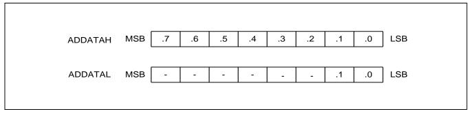
Figure 16-3 A/D Converter Data Register (ADDATAH/L)
