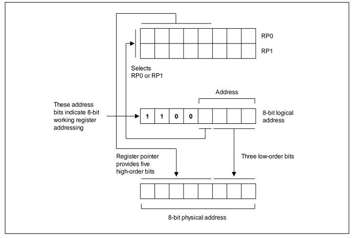
*Figure 2-14* illustrates the 8-bit working register addressing.
