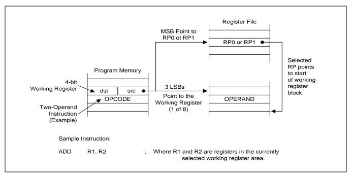
Figure 3-2 Working Register Addressing
