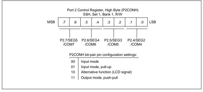
Figure 9-6 Port 2 High-Byte Control Register (P2CONH)
