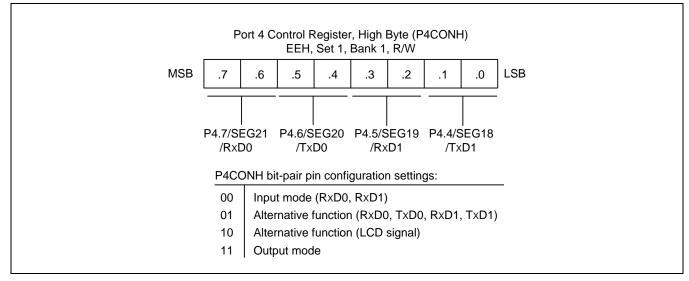
Figure 9-14 Port 4 High-Byte Control Register (P4CONH)
