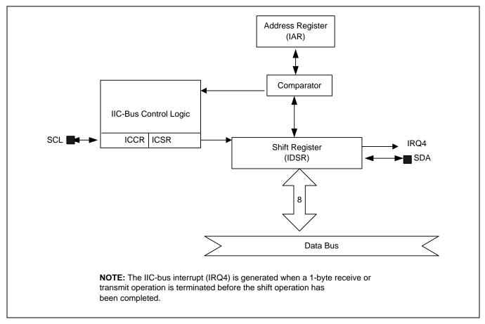
Figure 18-5 I2C Bus Block Diagram
