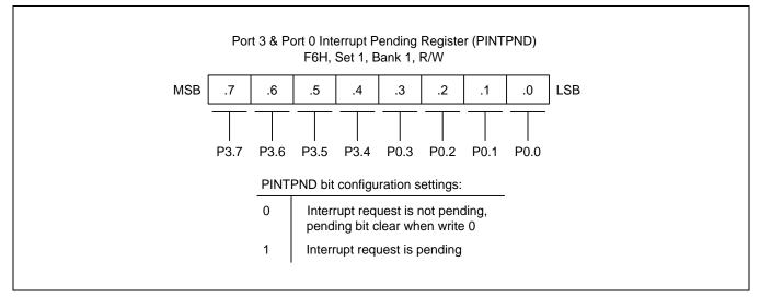
Figure 9-11 Port 3 and Port 0 Interrupt Pending Register (PINTPND)
