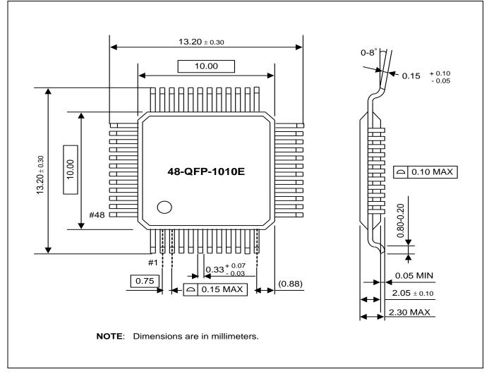
Figure 24-1 48-QFP-1010E Package Dimensions
