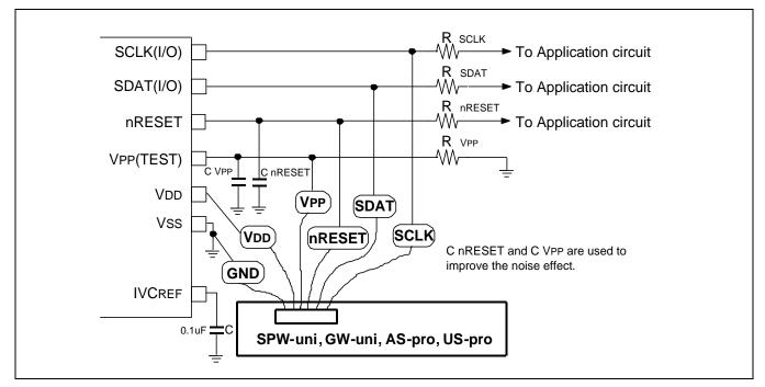
*Figure 25-3* illustrates the PCB design guide for on board programming.
