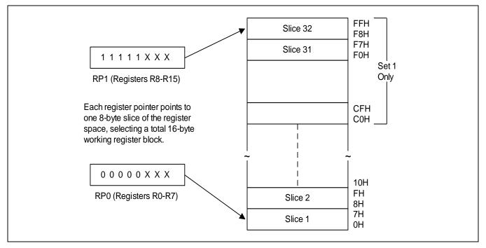
Figure 2-6 8 Byte Working Register Areas (Slices)
