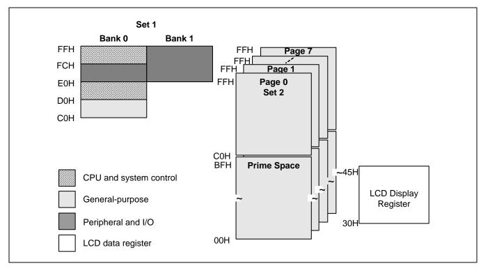
*Figure 2-5* illustrates the set 1, set 2, prime area register map, and LCD data register map.
