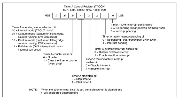
Figure 11-1 Timer A Control Register (TACON)
