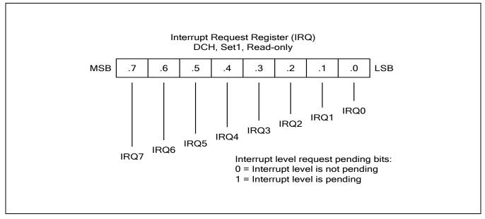
Figure 5-9 Interrupt Request Register (IRQ)
