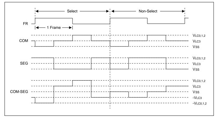
Figure 15-9 Select/No-Select Signal in 1/2 Duty, 1/2 Bias Display Mode
