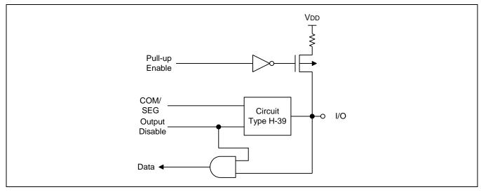
Figure 1-8 Pin Circuit Type H-44 (P2)
