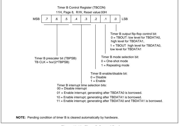
Figure 13-10 Timer B Control Register
