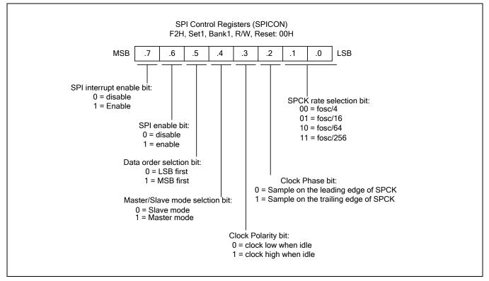
Figure 17-3 SPI Control Register (SPICON)
