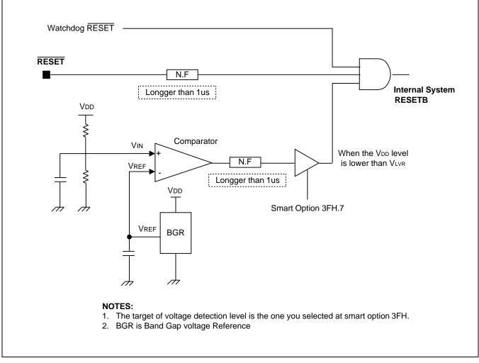
Figure 8-1 Low Voltage Reset Circuit
