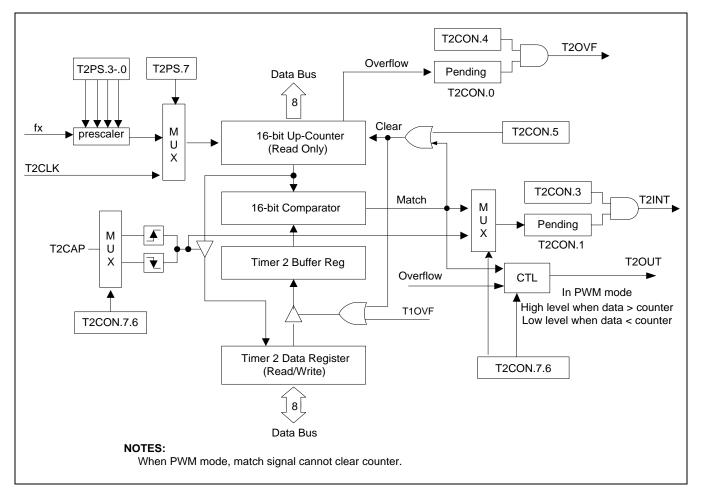
Figure 13-9 illustrates the functional block diagram of Timer 2.
