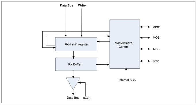
Figure 17-1 SPI Block Diagram
