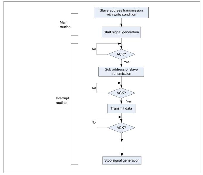
Figure 18-11 Write Operation Sequence
