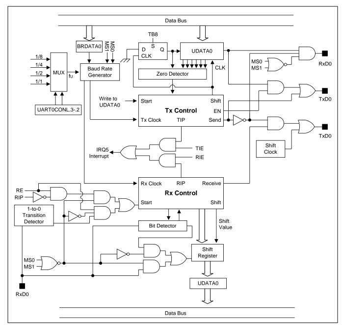
Figure 19-5 illustrates the functional block diagram of UART 0.
