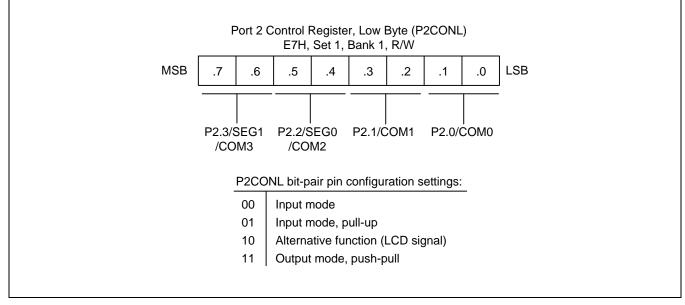
Figure 9-7 Port 2 Low-Byte Control Register (P2CONL)
