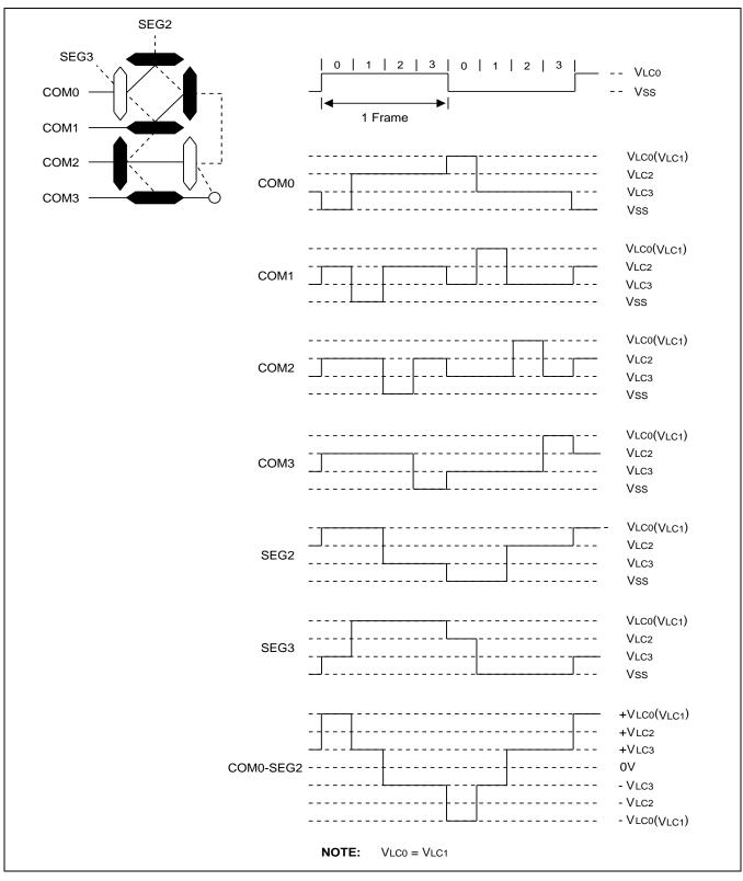
*Figure 15-13* illustrates the LCD signal waveforms (1/4 Duty, 1/3 Bias).
