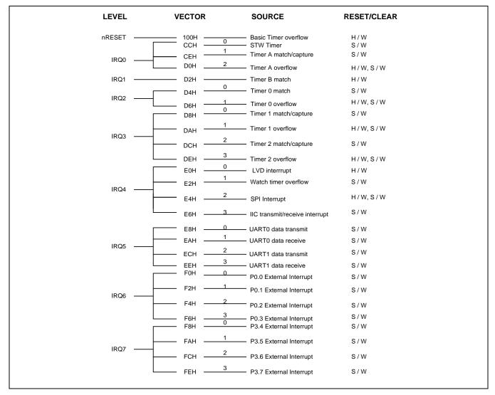
*Figure 5-2* illustrates the S3F8S19/S3F8S15 interrupt structure.
