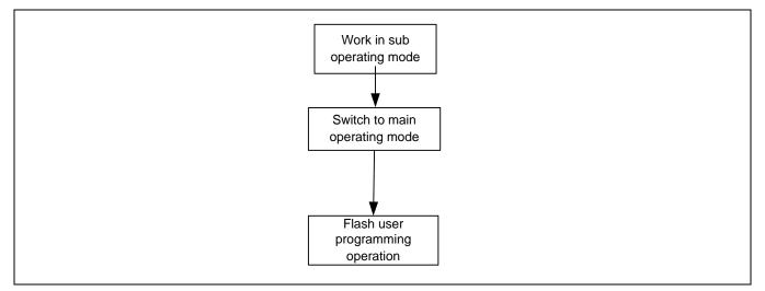
Figure 21-7 Flash Operation Sequence in Sub Operating Mode
