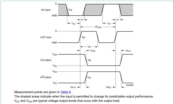
Fig. 7. Clock pulse width, maximum frequency, set-up times, hold times and input to output propagation delays
