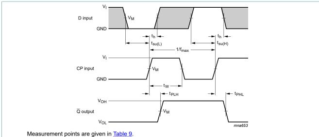
Logic levels:  $V_{OL}$  and  $V_{OH}$  are typical output voltage drop that occur with the output load.
