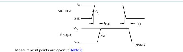
$V_{\text{OL}}$  and  $V_{\text{OH}}$  are typical output voltage levels that occur with the output load.
