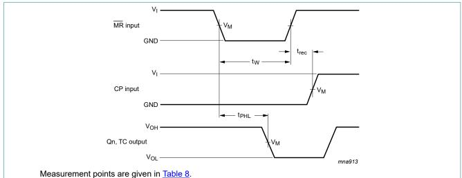
$V_{OL}$  and  $V_{OH}$  are typical output voltage levels that occur with the output load.
