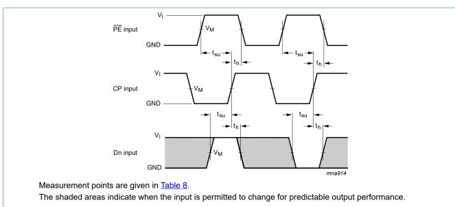
Fig. 12. Set-up and hold times for the input (Dn) and parallel enable input (PE)
