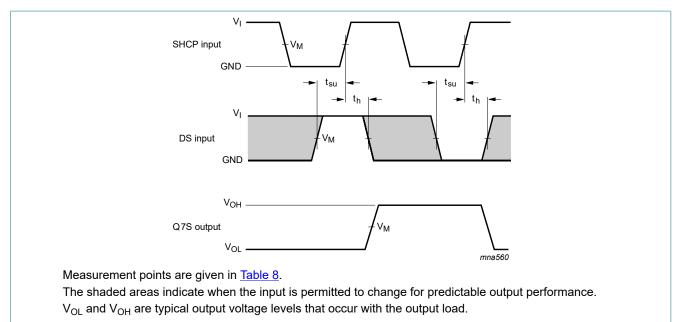
Fig. 9. The data set-up and hold times for the serial data input (DS)
