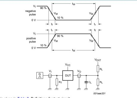
Test data is given in <u>Table 9</u>. Definitions for test circuit:
