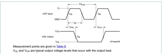
Fig. 6. Clock input (nCP) to output (nQn) propagation delay, the clock pulse width, and the maximum frequency
