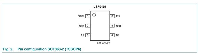
1-bit bidirectional multi-voltage level translator; open-drain; push-pull
