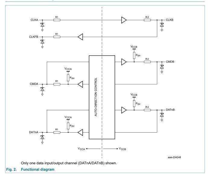
SD 3.0-compatible memory card integrated auto-direction control and level translator with EMI filter and ESD protection
