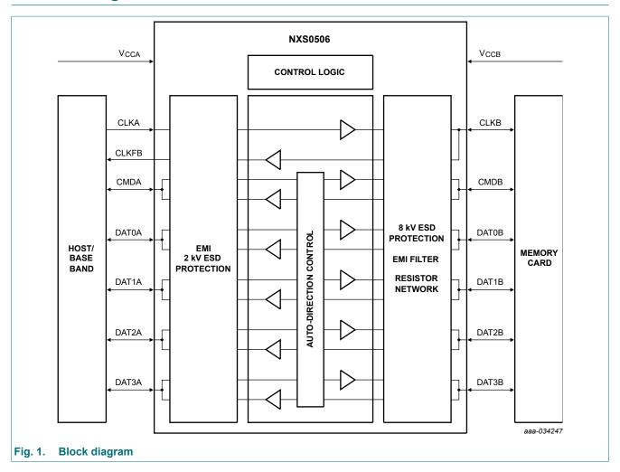
SD 3.0-compatible memory card integrated auto-direction control and level translator with EMI filter and ESD protection
