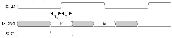
Table 89. Reduced Media Independent Interface (RMII) Clock Timing Requirements for Intel Stratix 10 Devices
