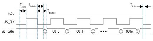
Figure 28. AS Configuration Serial Input Timing Diagram
