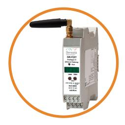
The IWR-PORT Ethernet Gateway provides a link between wireless sensors and sensor networks and Industrial Ethernet or RS-232/485 networks.
