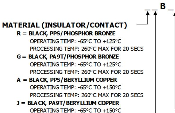
PROCESSING TEMP: 260°C MAX FOR 20 SECS
