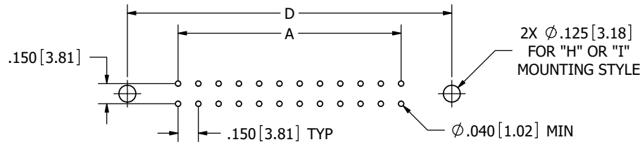
RECOMMENDED PCB LAYOUT
