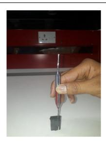
3. Insert the contact carefully and straight into the cable side of the connector until it snaps firmly into place.
