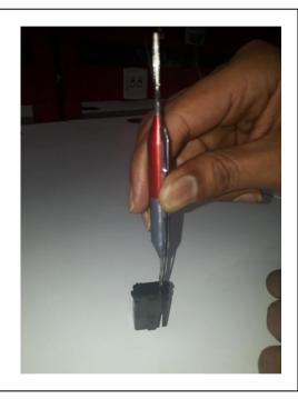
1. Insert the cable from the center of the tool into the groove of the white side.
