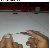
1. Place the cable on the groove and press from the center of the tool so that the contact remains outside
