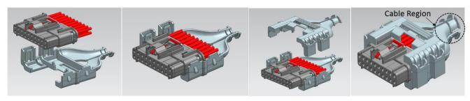
Above illustration shows the assembly with Receptacle housing and backshells. Same applies to Plug housing.
