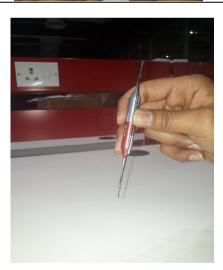
Using the cable, pull the contact firmly into the tool tip until the crimp pot of the contact is firmly seated in the tool tip.
