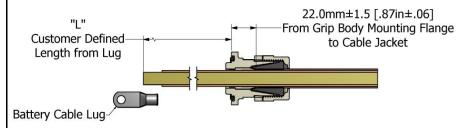
b) Slide the Compression Nut and Grommet onto the Cable Jacket
