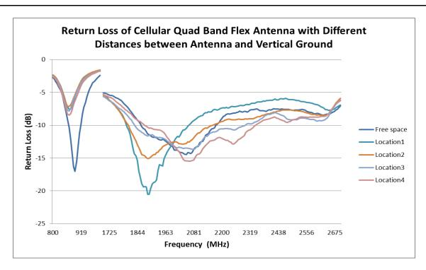
FIGURE 4.1.1 RETURN LOSS OF ANTENNA AT FOUR LOCATIONS WITH VERTICAL GROUND
