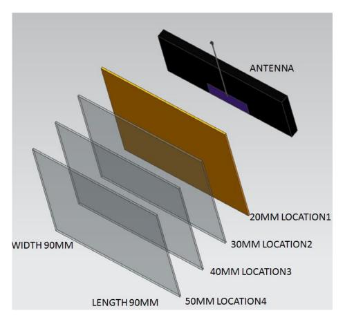
FIGURE 4.2 FOUR LOCATIONS WITH PARALLEL GROUND
