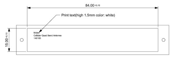
FIGURE 1. DIMENSION OF CELLULAR QUAD BAND FLEX ANTENNA
