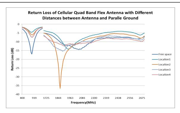
FIGURE 4.2.1 RETURN LOSS OF ANTENNA AT FOUR LOCATIONS WITH PARALLEL GROUND
