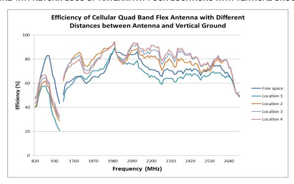
FIGURE 4.1.2 EFFICIENCY OF ANTENNA AT FOUR LOCATIONS WITH VERTICAL GROUND
