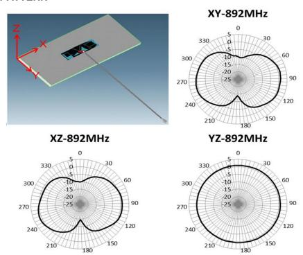
FIGURE 5.1 RADIATION PATTERN OF ANTENNA AT 892MHZ IN FREE SPACE
