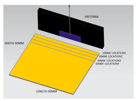
FIGURE 4.1 FOUR LOCATIONS WITH VERTICAL GROUND
