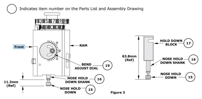
**Note:** The above dimensions were measured during setup and are included as a reference only. Additional adjustments may be required before crimping for production.
