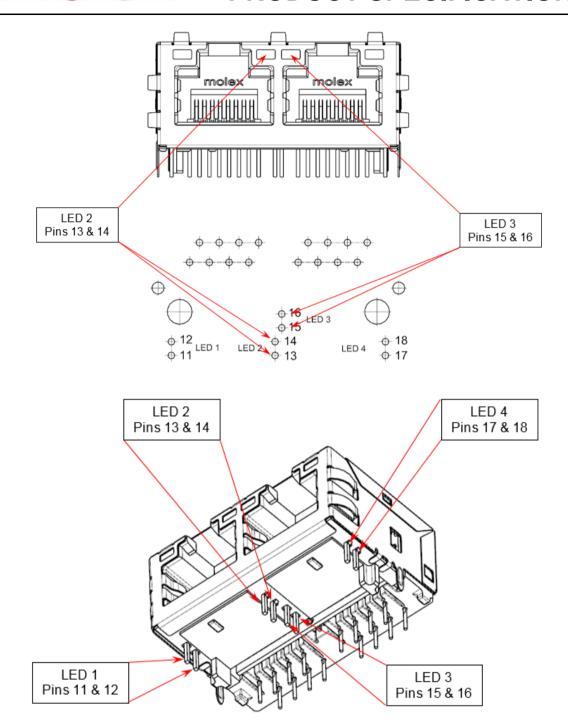
Figure 4: 0.85" Dual Port Inverted Connector LED Pin-out example
