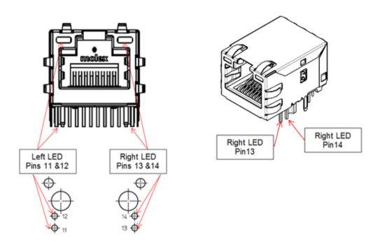
Figure 1: 0.85" Inverted Connector LED Pin-out example
