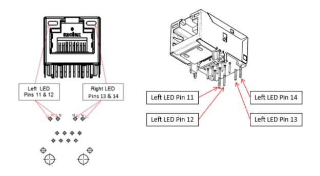
Figure 2: 1" Inverted Connector LED Pin-out example
