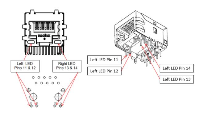
Figure 3: 0.85" Standard Connector LED Pin-out example
