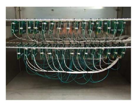
Connectors Mated and In Test Chamber
