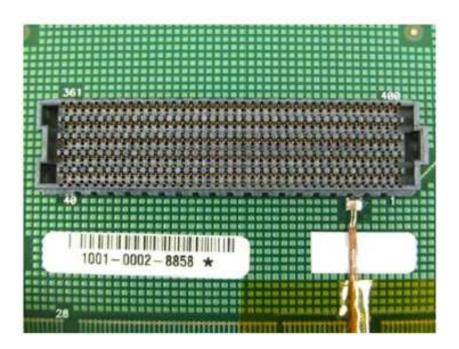
Figure 6: PCTB #186B w/ mounted Receptacle Connector
