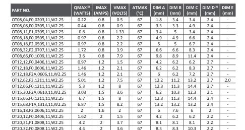
Notes: 1) QMax rated value at  $\Delta T = 0$ °C, Imax and Vmax, Th = 25°C; 2) Thickness for non-metallized versions only. All modules are lead-free. For wiring options contact Laird.
