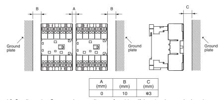
\*3. Set dimension C to an adequate distance for wiring. If the wires have to be bent in a small space, check the minimum bending dimensions with the wire manufacturer before connecting the wiring.
