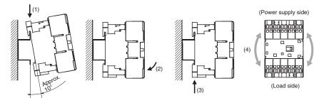
When mounting on a rail, use the end plate.
