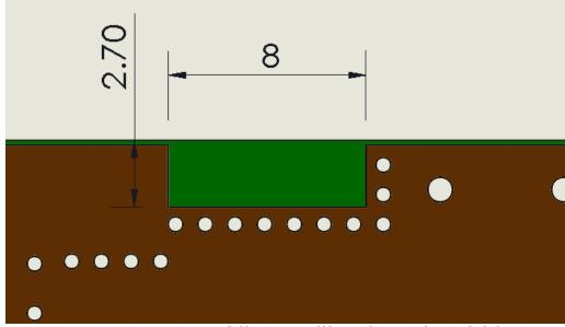
\*Clearance 8mm × 2.7mm : All metallization should be removed from all PCB layers.
