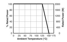
Derating (thermal resist.) 66.6 W/K (0.015 K/W) Power rating: 2,000 W at 125°C bottom case temperature
