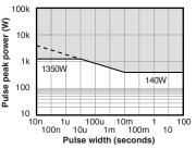
Tentative continuous-pulse power allowance at duty 0.01. Load life test will be necessary in actual equipment, Because curve will be changed by resistance, repetition, duty and operating tempera-ture. Dotted is estimation.
