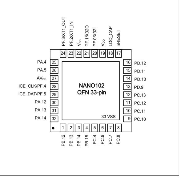
Figure 4-4 NuMicro<sup>™</sup> Nano102 QFN 32-pin Diagram
