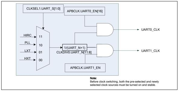
Figure 6-52 UART Clock Control Diagram
