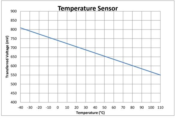
Figure 6-129 Temperature Sensor Transfer Function
