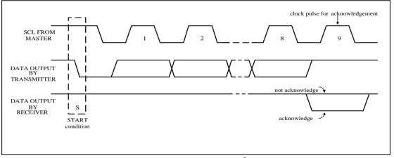
Figure 6-78 Acknowledge on I<sup>2</sup>C Bus
