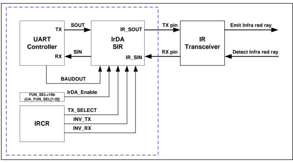
Figure 6-61 IrDA Block Diagram
