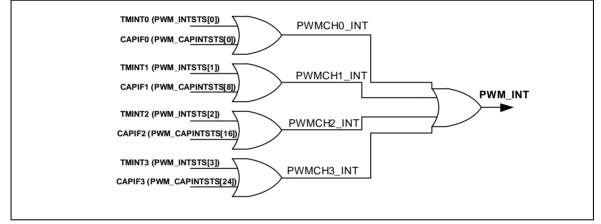
Figure 6-44 PWM-Timer Interrupt
