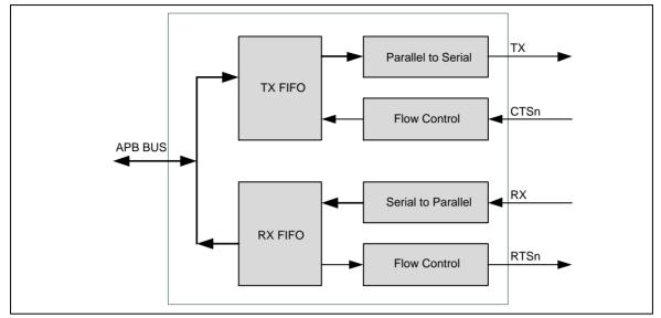
Figure 6-55 UART Auto-Flow Control Block Diagram
