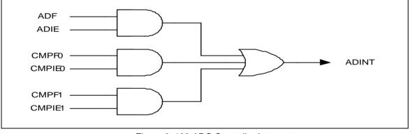
Figure 6-123 ADC Controller Interrupt
