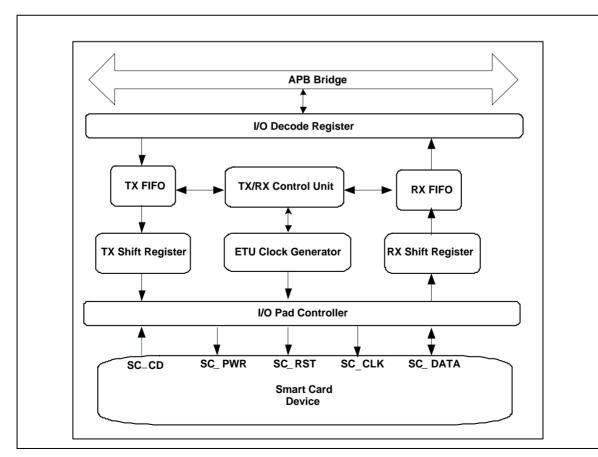
Figure 6-67 SC Controller Block Diagram
