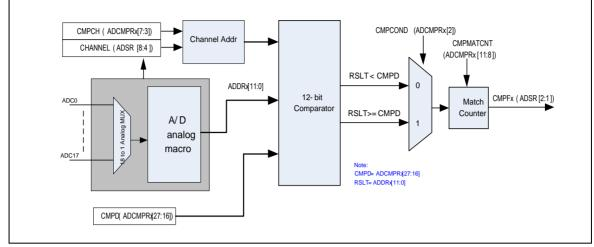
Figure 6-122 ADC Conversion Result Monitor Logic Diagram
