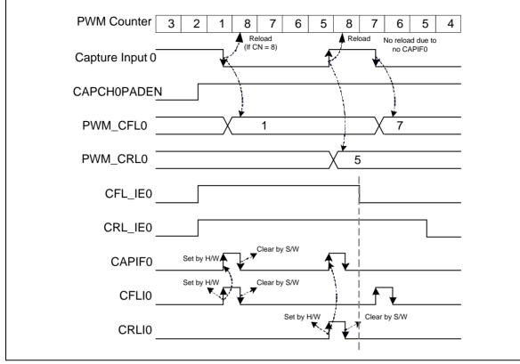
Figure 6-43 PWM Capture Operation Timing
