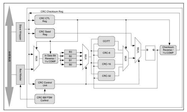
Figure 6-27 CRC Generator Block Diagram
