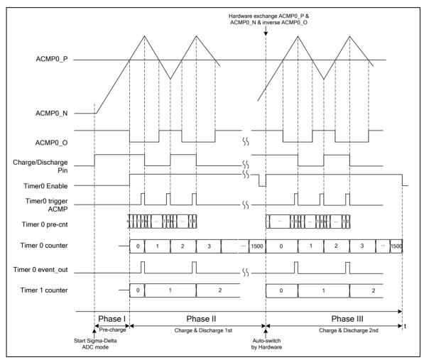
Figure 6-137 ACMP Sigma-Delta ADC Mode Timing
