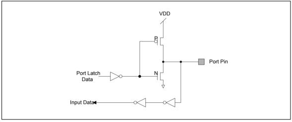
Figure 6-23 Push-Pull Output
