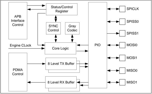
Figure 6-88 SPI Block Diagram
