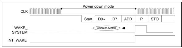
Figure 6-60 UART RS-485 AAD Mode Address Match Wake-Up
