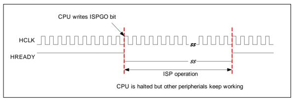
Figure 6-20 CPU Halt during ISP Operation
