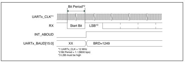
Figure 6-54 UART Auto-Baud Rate Block Diagram
