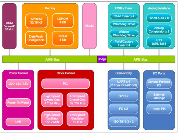
Figure 5-2 NuMicro<sup>™</sup> Nano112 Block Diagram
