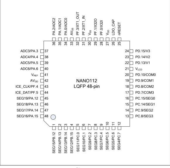
Figure 4-7 NuMicro<sup>™</sup> Nano112 LQFP 48-pin Diagram
