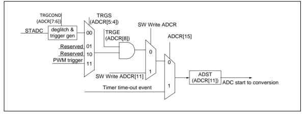
Figure 6-124 ADC Start Conversion Conditions
