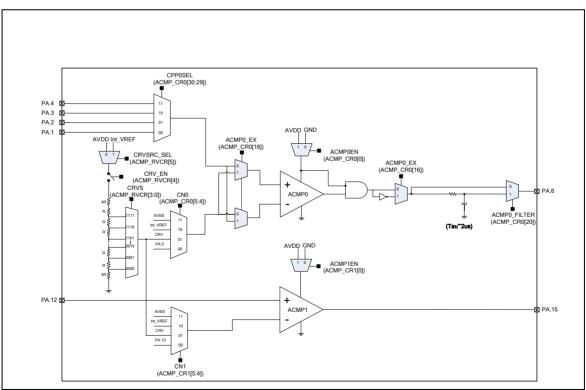
Figure 6-133 Normal Comparator Mode Block Diagram
