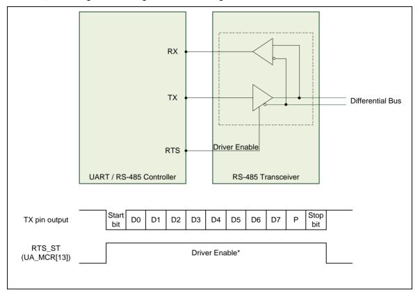
Figure 6-63 Structure of RS-485 Frame
