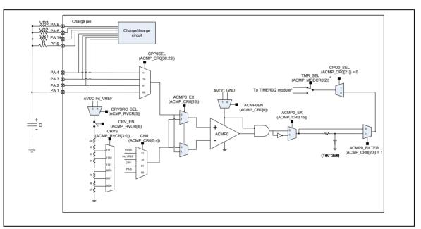
Figure 6-134 ACMP Single Slope ADC Mode Reference Circuit
