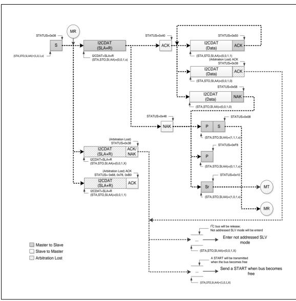
Figure 6-83 Master Receiver Mode Control Flow
