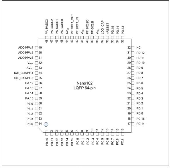
Figure 4- 2 NuMicro<sup>™</sup> Nano102 LQFP 64-pin Diagram
