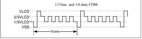
Figure 6-106 COM Signal Waveform
