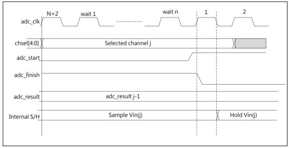
Figure 6-126 Increased Sampling Time Waveform
