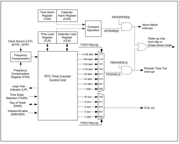
Figure 6-51 RTC Core Block Diagram
