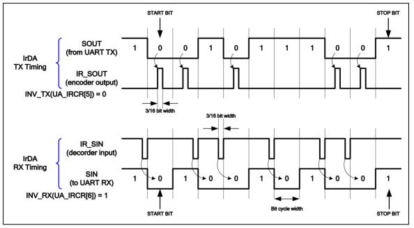
Figure 6-62 IrDA TX/RX Timing Diagram
