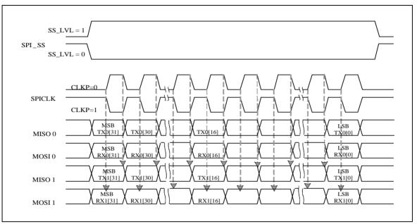
Figure 6-96 SPI 2-bit Transfer Mode Timing Diagram
