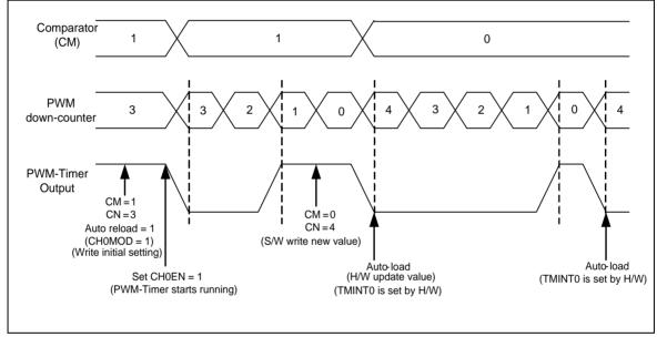
Figure 6-37 Legend of Internal Comparator Output of PWM-Timer
