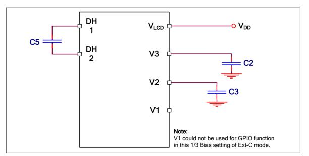
Figure 6-64 1/3 Bias (External Capacitor Ladder)
