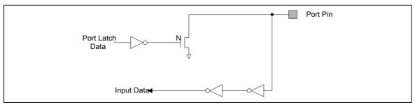
Figure 6-24 Open-Drain Output
