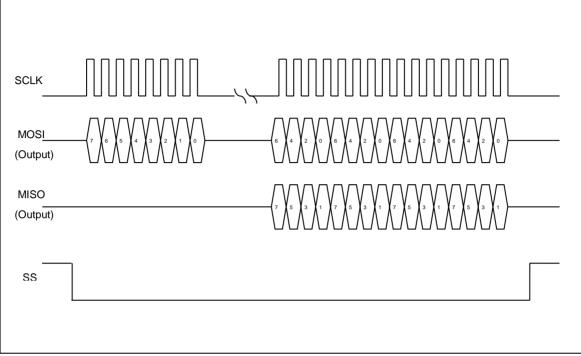
Figure 6-97 SPI DUAL-I/O output Sequence
