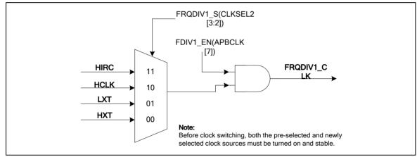
Figure 6-10 Clock Source of Frequency Divider1
