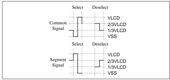
Figure 6-107 SEG Signal Waveform
