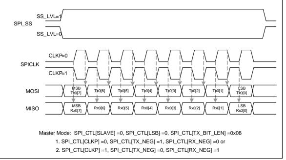
Figure 6-99 SPI Timing in Master Mode
