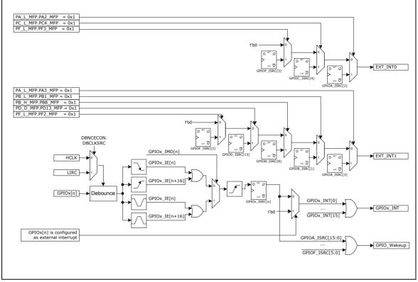
Figure 6-22 GPIO Block Diagram
