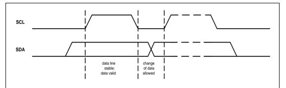
Figure 6-77 Bit Transfer on I<sup>2</sup>C Bus
