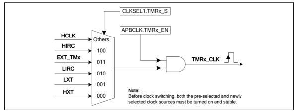
Figure 6-30 Timer Clock Controller Diagram
