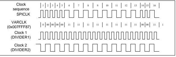
Figure 6-91 SPI Variable Clock Frequency
