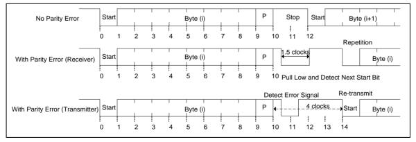
Figure 6-73 SC Error Signal
