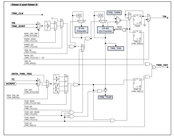
Figure 6-29 Timer 1 and Timer 3 Controller Block Diagram
