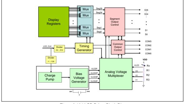
Figure 6-104 LCD Driver Block Diagram
