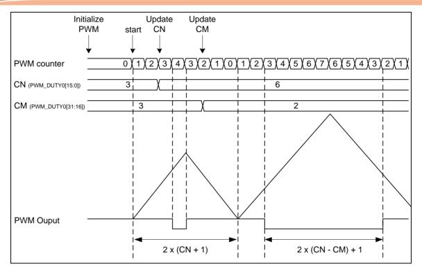
Figure 6-39 PWM-Timer Operation in Center-aligned Mode
