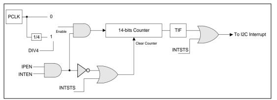
Figure 6-79 I<sup>2</sup>C Time-out Block Diagram
