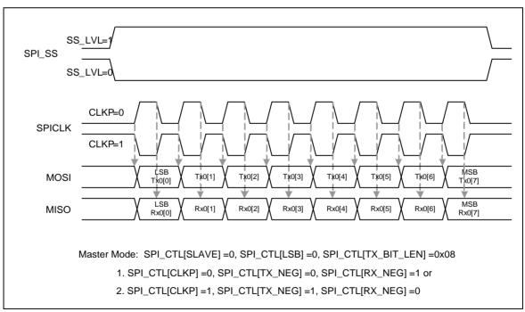
Figure 6-100 SPI Timing in Master Mode (Alternate Phase of SPICLK & LSB = 1)
