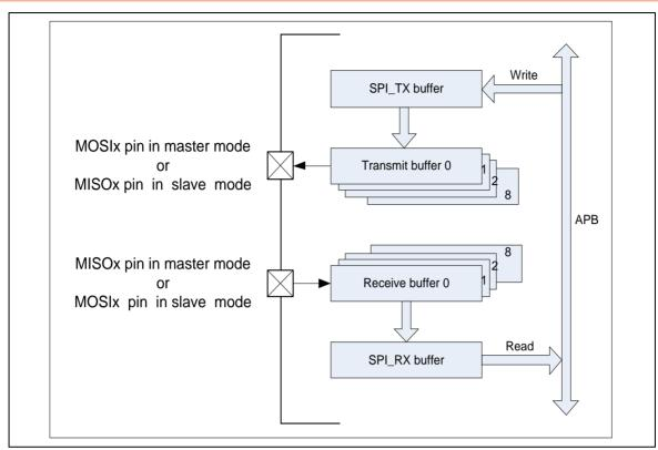
Figure 6-98 SPI FIFO Mode Control
