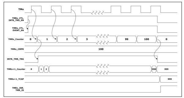
Figure 6-32 Inter-Timer Trigger Mode
