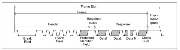
Figure 6-64 Structure of LIN Frame
