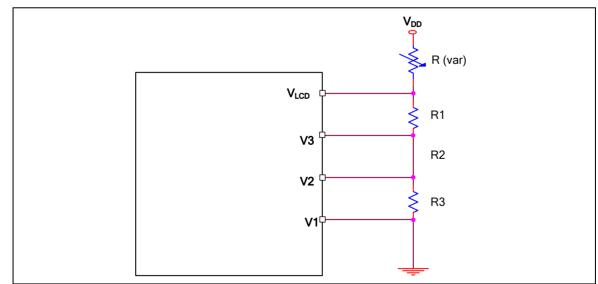
Figure 6-110 1/2 Bias (External Resistor Ladder)
