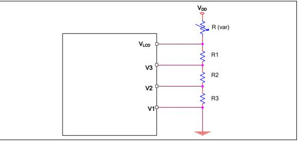
Figure 6-109 1/3 Bias (External Resistor Ladder)
