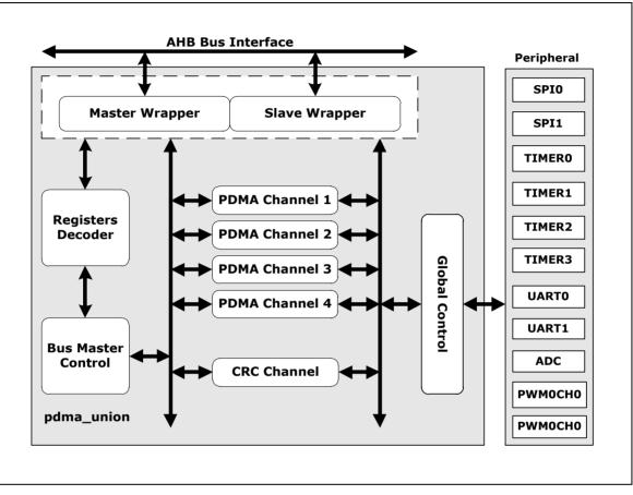
Figure 6-25 DMA Controller Block Diagram
