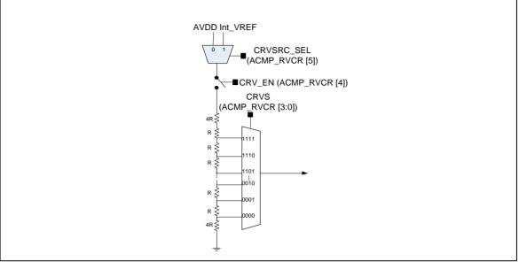
Figure 6-132 Comparator Reference Voltage Block Diagram
