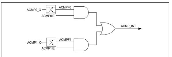
Figure 6-138 Analog Comparator Interrupt Sources
