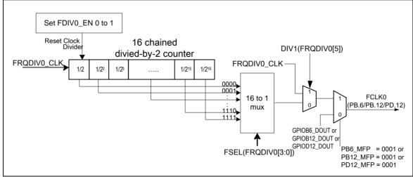
Figure 6-11 Frequency Divider0 Block Diagram
