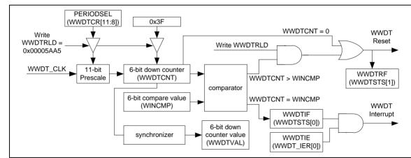
Figure 6-49 Window Watchdog Controller Block Diagram
