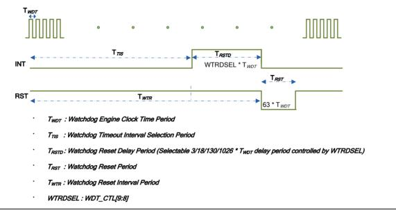
Figure 6-48 Watchdog Timing of Interrupt and Reset Signal
