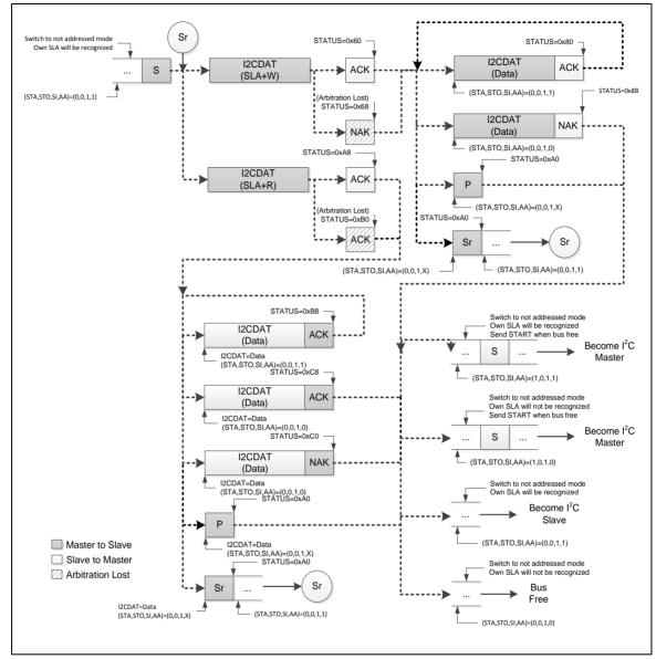
Figure 6-84 Slave Mode Control Flow
