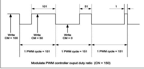
Figure 6-41 PWM Controller Output Duty Ratio
