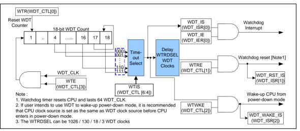
Figure 6-46 Watchdog Controller Block Diagram
