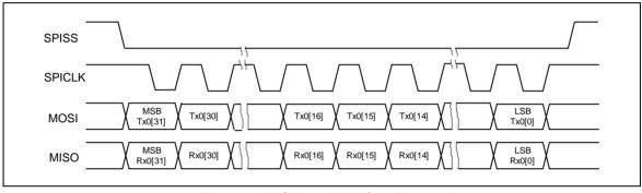
Figure 6-92 SPI 32-bit in One Transaction
