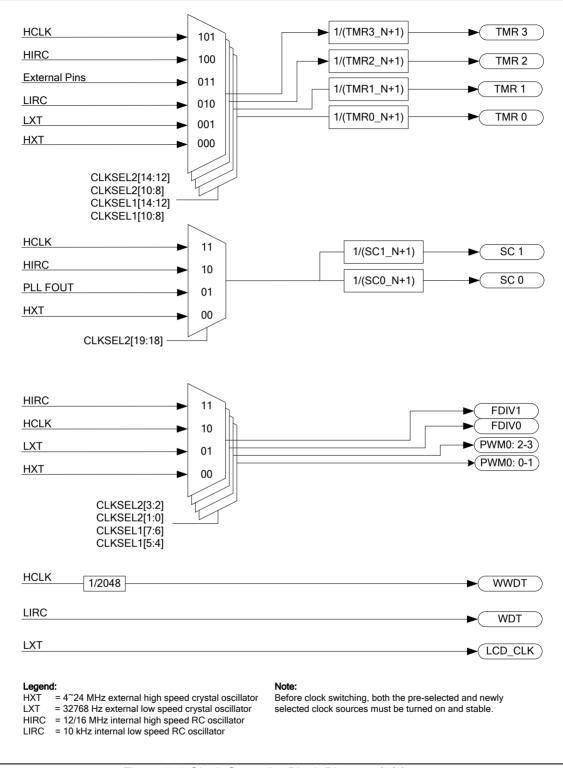
Figure 6-8 Clock Controller Block Diagram (3/3)
