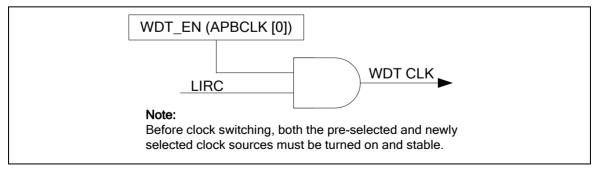
Figure 6-47 Watchdog Timer Clock Control Diagram
