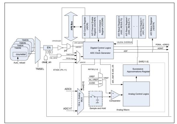
Figure 6-117 ADC Controller Block Diagram
