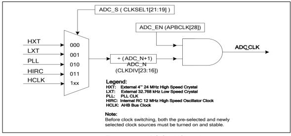
Figure 6-118 ADC Clock Control
