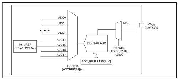
Figure 6-130 Int\_V<sub>REF</sub> for Measuring AV<sub>DD</sub> Application Block Diagram
