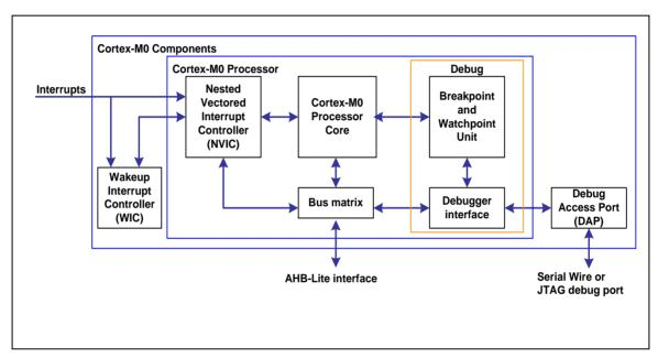
Figure 6-1 Functional Block Diagram
