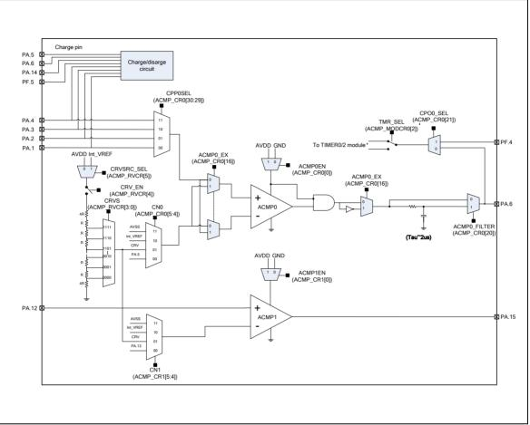
Figure 6-131 Analog Comparator Block Diagram
