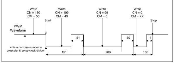
Figure 6-40 PWM Double Buffer Illustration
