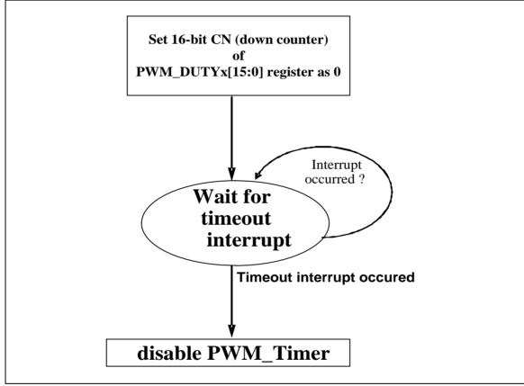
Figure 6-45 PWM-Timer Stop Method 1
