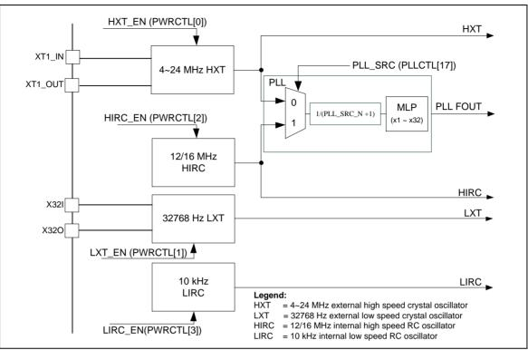
Figure 6-6 Clock Controller Block Diagram (1/3)
