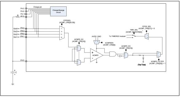
Figure 6-136 ACMP Sigma-Delta ADC Mode Reference Circuit
