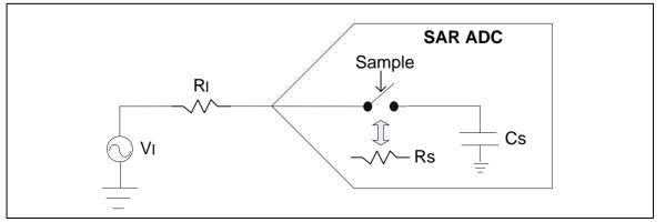
Figure 6-125 Model of Sampling Network
