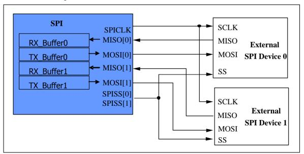
Figure 6-95 SPI 2-bit Transfer Mode
