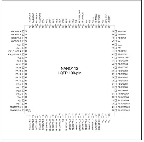
Figure 4-5 NuMicro<sup>™</sup> Nano112 LQFP 100-pin Diagram
