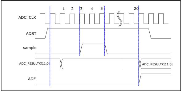
Figure 6-119 ADC Single Mode Conversion Timing Diagram
