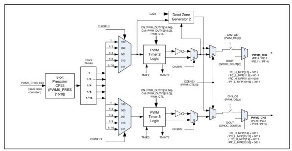
Figure 6-36 PWM Generator for Channel 2, 3
