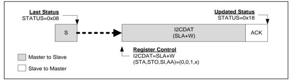
Figure 6-81 Control I2C Bus according to Current I<sup>2</sup>C Status
