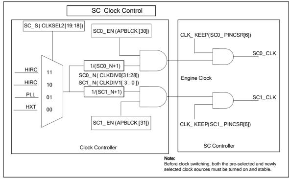
Figure 6-66 SC Clock Control Diagram (4-bit Prescale Counter in Clock Controller)
