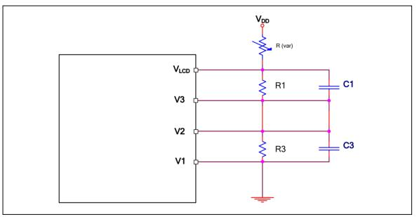
Figure 6-112 1/2 Bias (Resistor Ladder with Capacitor)
