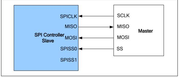
Figure 6-90 SPI Slave Mode Application Block Diagram
