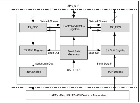
Figure 6-53 UART Block Diagram
