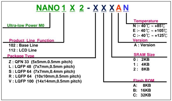
Figure 4-1 NuMicro<sup>™</sup> Nano112 Series Selection Code
