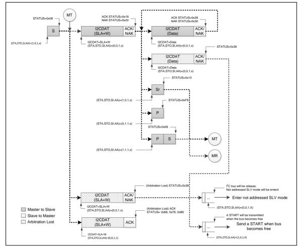
Figure 6-82 Master Transmitter Mode Control Flow
