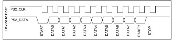
Figure 6-90 Data Format of Device-to-Host
