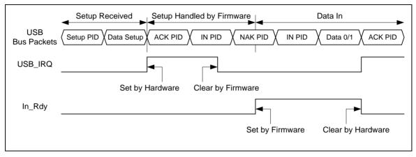
Figure 6-139 Setup Transaction Followed by Data IN Transaction
