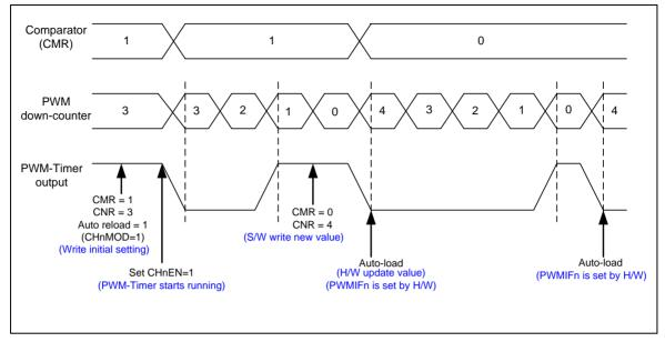
Figure 6-39 PWM-Timer Operation Timing
