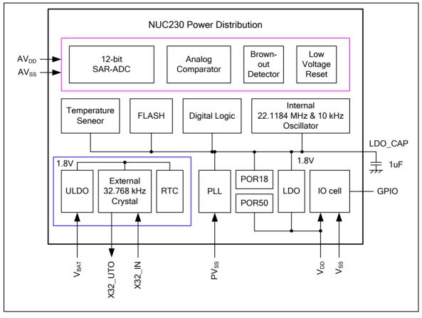
Figure 6-2 NuMicro™ NUC230 Power Distribution Diagram
