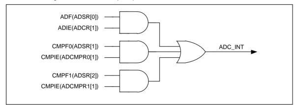
Figure 6-159 A/D Controller Interrupt
