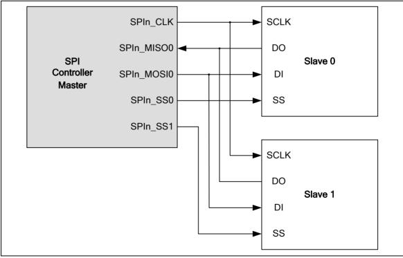
Figure 6-114 SPI Master Mode Application Block Diagram
