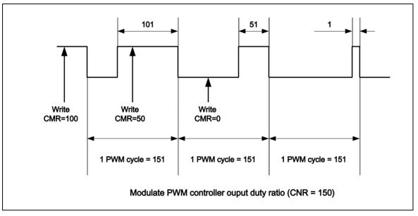
Figure 6-44 PWM Controller Output Duty Ratio
