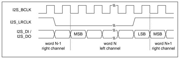
Figure 6-130 I<sup>2</sup>S Data Format Timing Diagram
