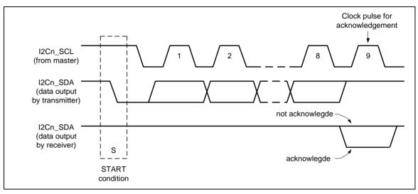
Figure 6-100 Acknowledge on the I<sup>2</sup>C Bus
