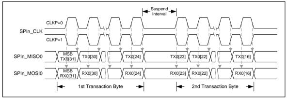
Figure 6-119 Timing Waveform for Byte Suspend
