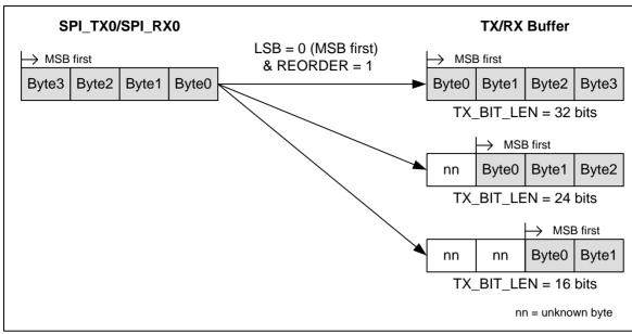
Figure 6-118 Byte Reorder Function
