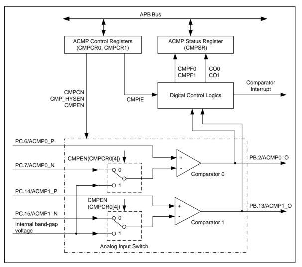
Figure 6-162 Analog Comparator Block Diagram
