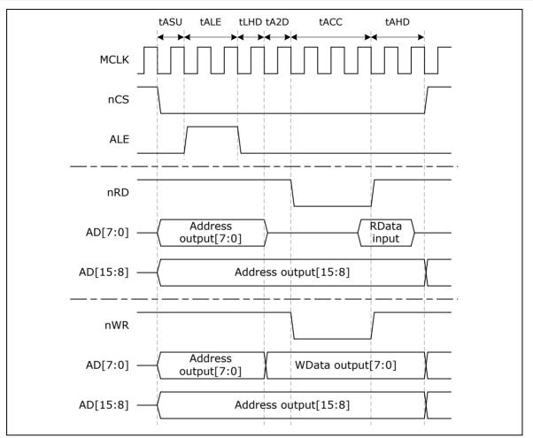
Figure 6-20 Timing Control Waveform for 8-bit Data Width
