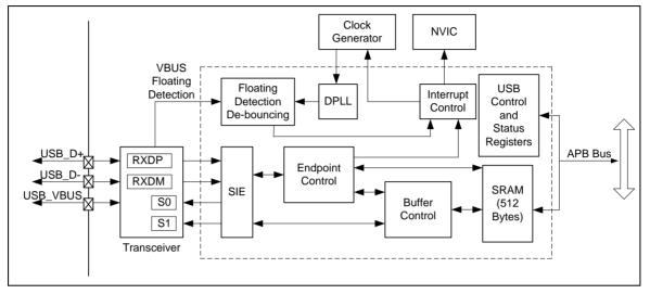
Figure 6-136 USB Device Block Diagram
