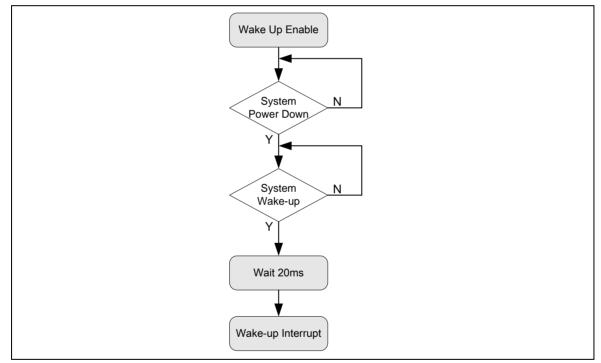
Figure 6-137 Wake-up Interrupt Operation Flow
