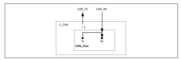
Figure 6-142 CAN Core in Silent Mode
