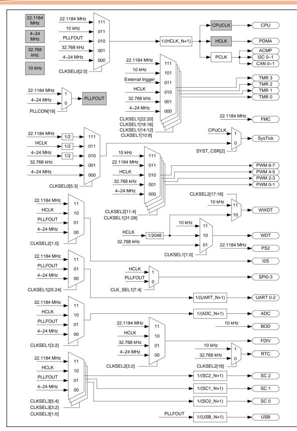
Figure 6-5 Clock Generator Global View Diagram
