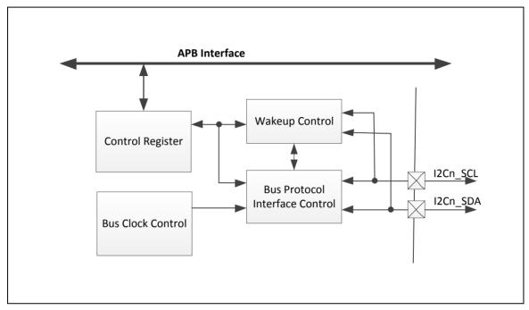
Figure 6-95 I<sup>2</sup>C Controller Block Diagram
