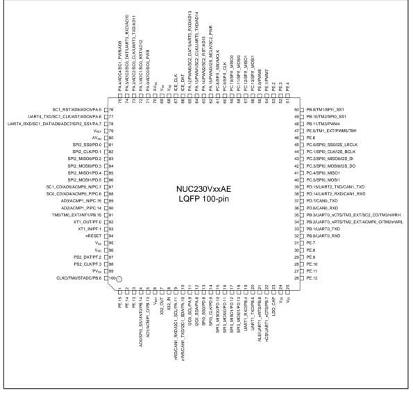
Figure 4-2 NuMicro™ NUC230VxxAE LQFP 100-pin Diagram
