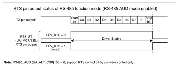
Figure 6-74 RS-485 RTS Driving Level with Software Control
