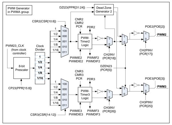
Figure 6-33 PWM Generator 2 Architecture Diagram
