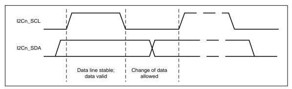
Figure 6-99 Bit Transfer on the I<sup>2</sup>C Bus
