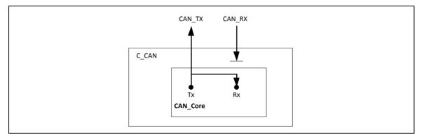
Figure 6-143 CAN Core in Loop Back Mode
