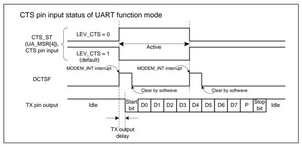
Figure 6-61 UART CTS Auto Flow Control Enabled
