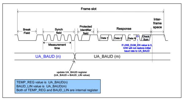
Figure 6-72 UA\_BAUD Update Sequence in Automatic Resynchronization Mode when LINS\_DUM\_EN (UA\_LIN\_CTL[3])= 0
