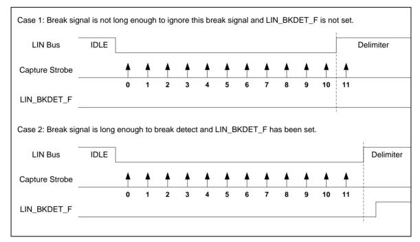
Figure 6-68 Break Detection in LIN Mode
