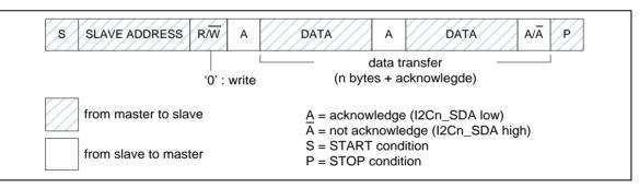
Figure 6-101 Master Transmits Data to Slave
