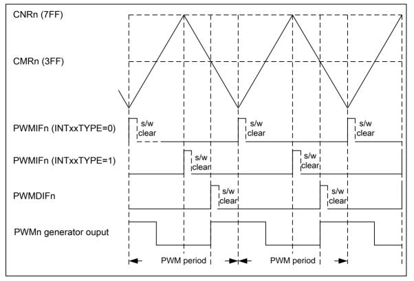
Figure 6-42 PWM Center-aligned Interrupt Generate Timing Waveform
