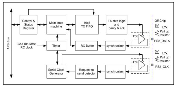
Figure 6-89 PS/2 Device Block Diagram
