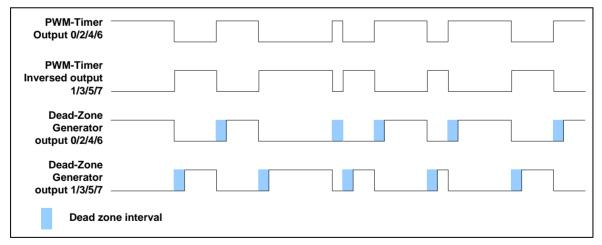
Figure 6-45 Paired-PWM Output with Dead-zone Generation Operation
