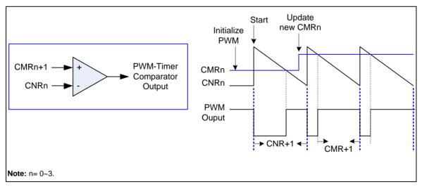
Figure 6-38 Legend of Internal Comparator Output of PWM-Timer
