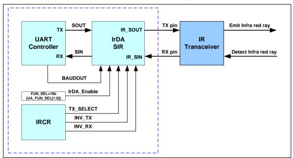
The following diagram demonstrates the IrDA control block diagram.
