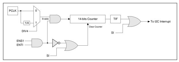
Figure 6-110 I<sup>2</sup>C Time-out Count Block Diagram
