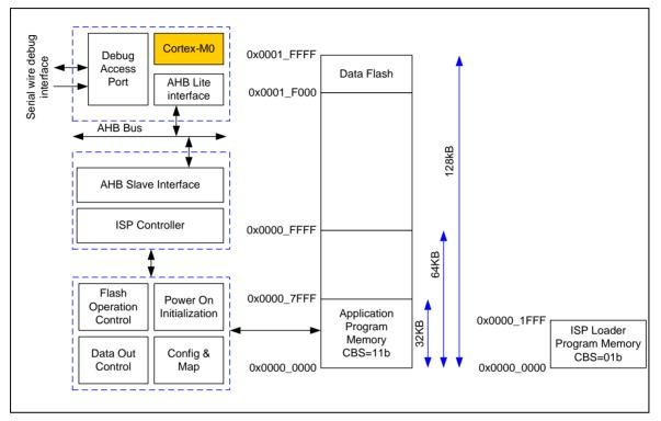
Figure 6-10 Flash Memory Control Block Diagram
