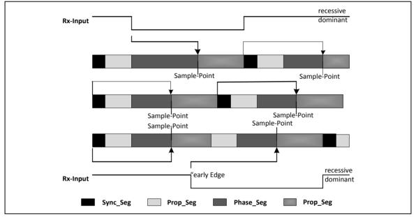
Figure 6-149 Synchronization on "late" and "early" Edges
