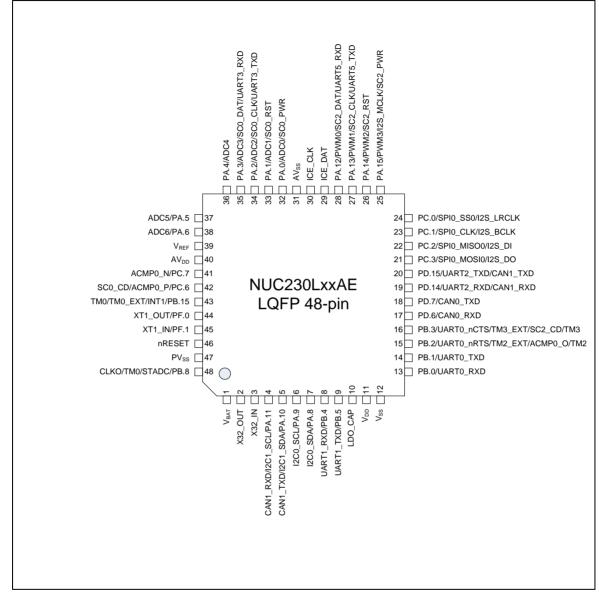
Figure 4-4 NuMicro™ NUC230LxxAE LQFP 48-pin Diagram
