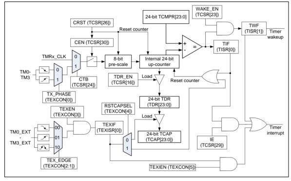
Figure 6-27 Timer Controller Block Diagram
