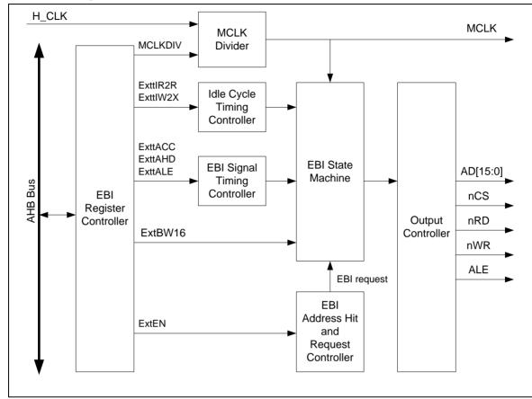
Figure 6-16 EBI Block Diagram
