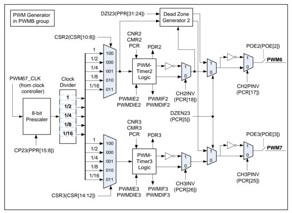
Figure 6-37 PWM Generator 6 Architecture Diagram
