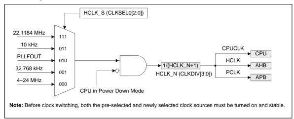
Figure 6-6 System Clock Block Diagram
