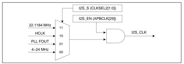
Figure 6-129 I<sup>2</sup>S Clock Control Diagram
