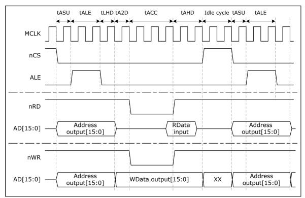
Figure 6-21 Timing Control Waveform for Insert Idle Cycle
