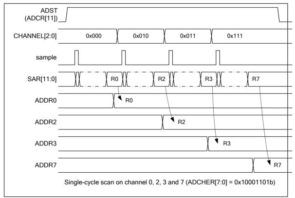
Figure 6-155 Single-Cycle Scan on Enabled Channels Timing Diagram
