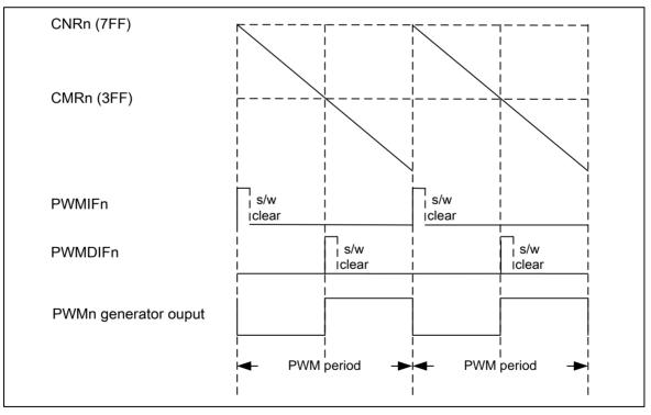
Figure 6-40 PWM Edge-aligned Interrupt Generate Timing Waveform
