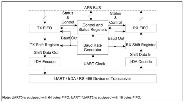
Figure 6-58 UART Block Diagram
