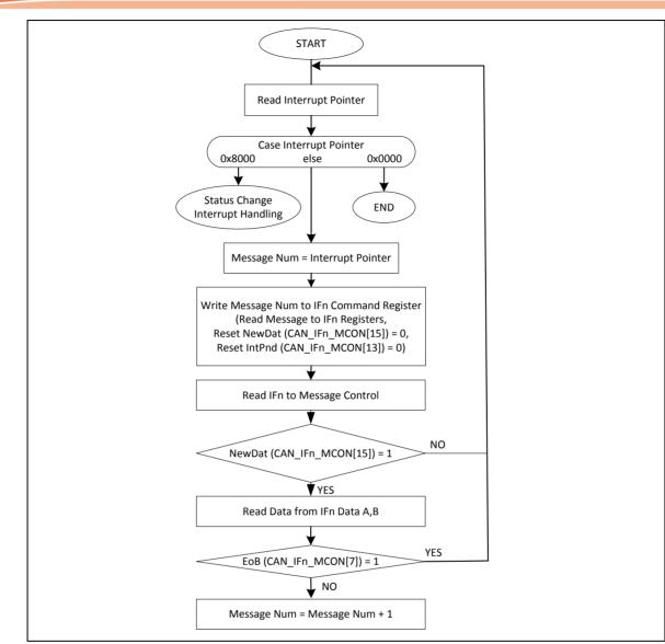
Figure 6-146 Application Software Handling of a FIFO Buffer
