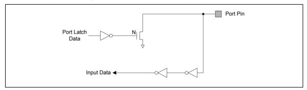
Figure 6-23 Open-Drain Output
