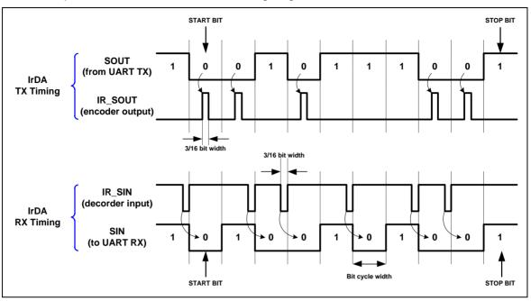
and half-duplex serial SIR interface. The following diagram is IrDA encoder/decoder waveform.
