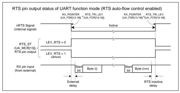
Figure 6-62 UART RTS Auto Flow Control Enabled
