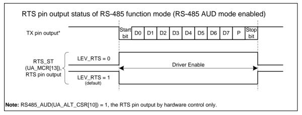
Figure 6-73 RS-485 RTS Driving Level in Auto Direction Mode
