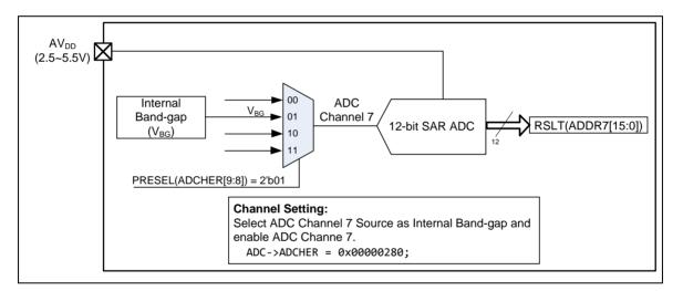
Figure 6-157 V<sub>BG</sub> for Measuring AV<sub>DD</sub> Application Block Diagram
