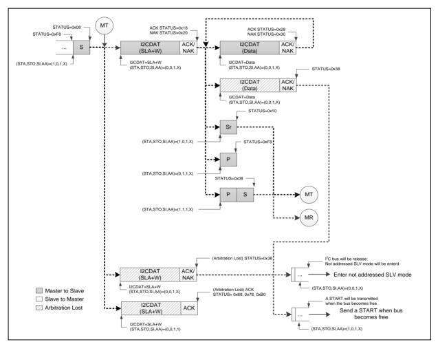
Figure 6-104 Master Transmitter Mode Control Flow
