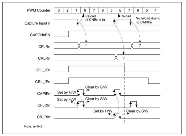
Figure 6-47 Capture Operation Timing
