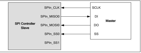
Figure 6-115 SPI Slave Mode Application Block Diagram
