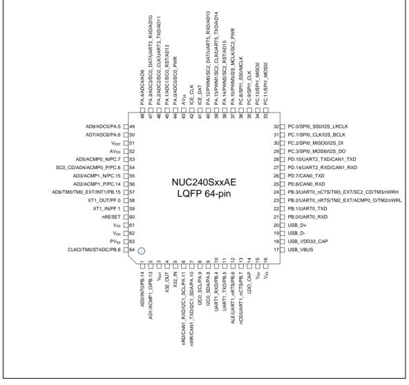
Figure 4-6 NuMicro™ NUC240SxxAE LQFP 64-pin Diagram
