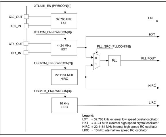
Figure 6-4 Clock Generator Block Diagram
