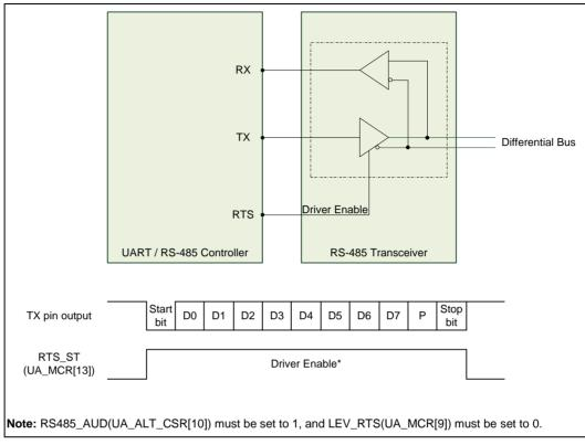
Figure 6-75 Structure of RS-485 Frame
