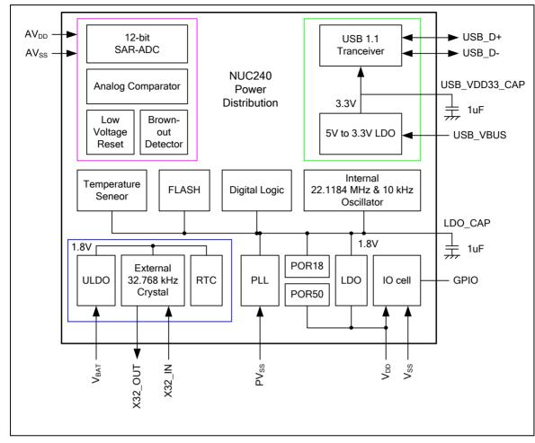
Figure 6-3 NuMicro™ NUC240 Power Distribution Diagram
