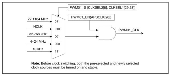
Figure 6-30 PWM Generator 0 Clock Source Control
