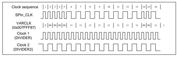
Figure 6-117 Variable Bus Clock Frequency
