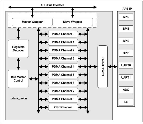
Figure 6-25 DMA Controller Block Diagram
