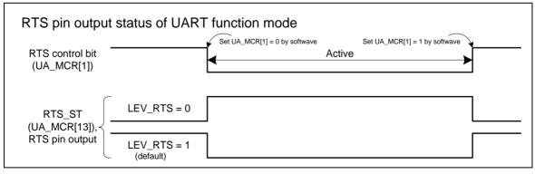
Figure 6-63 UART RTS Flow with Software Control
