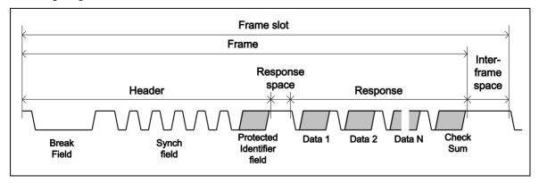
Figure 6-66 Structure of LIN Frame
