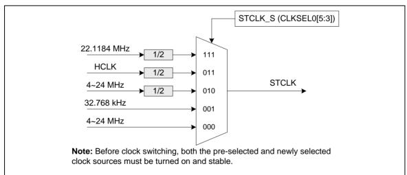
Figure 6-7 SysTick Clock Control Block Diagram
