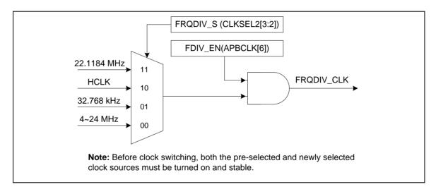
Figure 6-8 Clock Source of Frequency Divider
