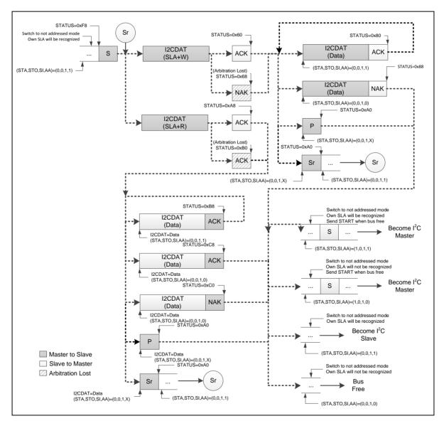
Figure 6-106 Save Mode Control Flow
