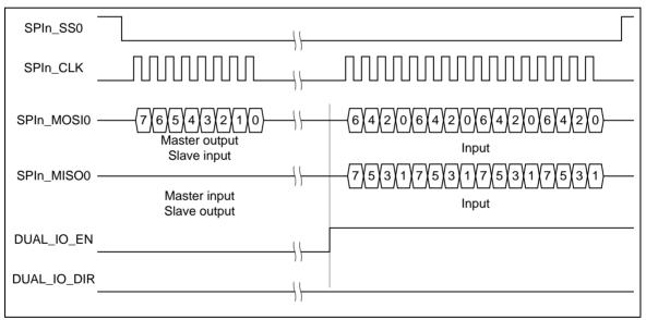
Figure 6-122 Bit Sequence of Dual Input Mode
