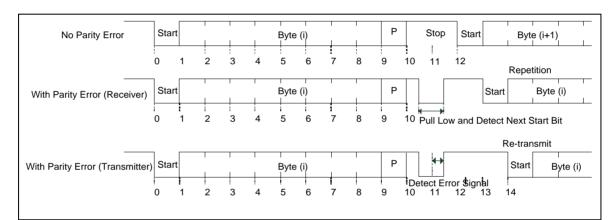
Figure 6-83 SC Error Signal
