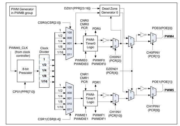
Figure 6-35 PWM Generator 4 Architecture Diagram
