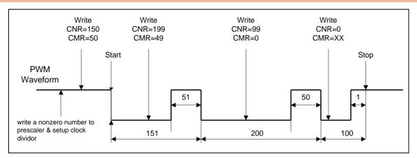
Figure 6-43 PWM Double Buffering Illustration
