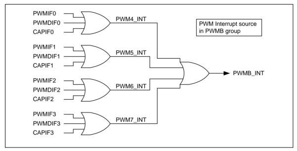
Figure 6-49 PWM Group B PWM-Timer Interrupt Architecture Diagram
