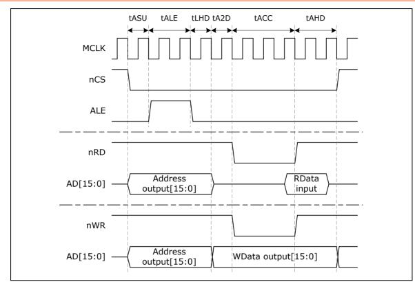
Figure 6-19 Timing Control Waveform for 16-bit Data Width
