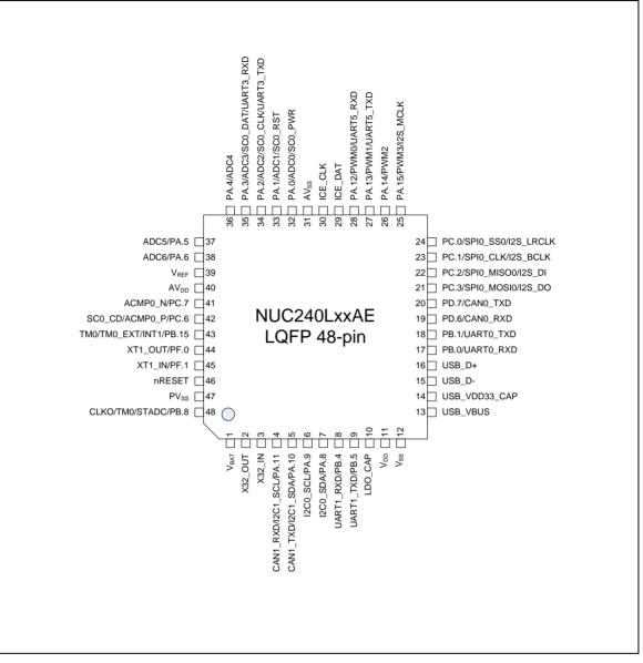
Figure 4-7 NuMicro™ NUC240LxxAE LQFP 48-pin Diagram
