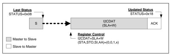
Figure 6-103 Control I<sup>2</sup>C Bus according to Current I<sup>2</sup>C Status
