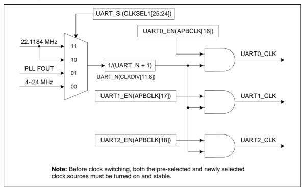
Figure 6-57 UART Clock Control Diagram
