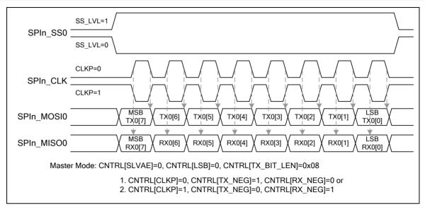
Figure 6-124 SPI Timing in Master Mode
