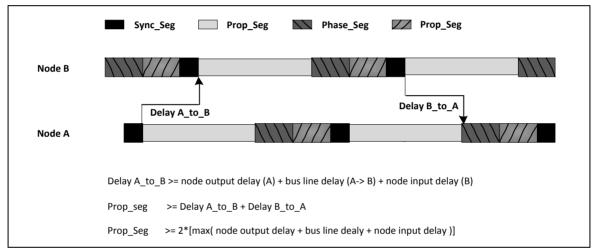
Figure 6-148 Propagation Time Segment
