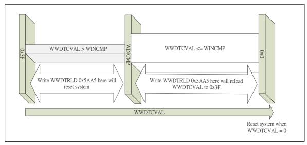
Figure 6-55 Window Watchdog Timer Reset and Reload Behavior
