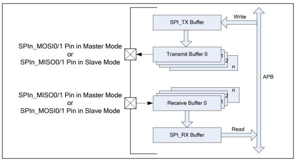
Figure 6-123 FIFO Mode Block Diagram
