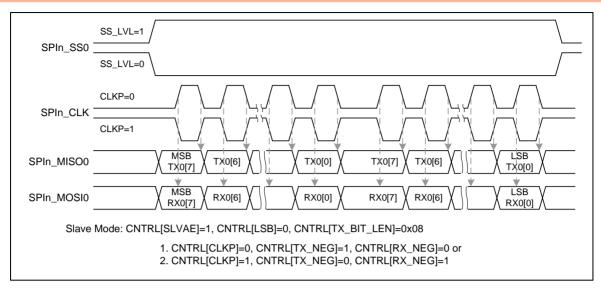
Figure 6-126 SPI Timing in Slave Mode
