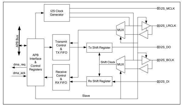
Figure 6-128 I<sup>2</sup>S Controller Block Diagram
