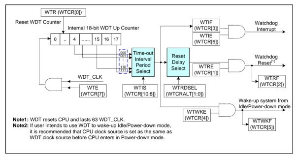
Figure 6-51 Watchdog Timer Block Diagram
