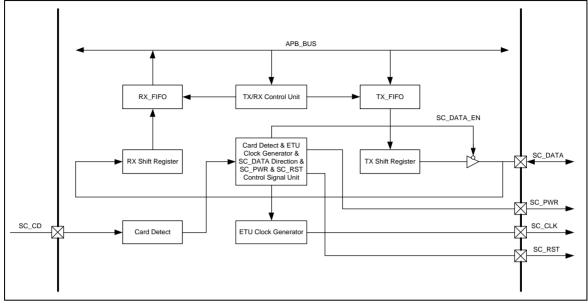
Figure 6-77 SC Controller Block Diagram
