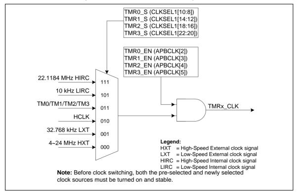
Figure 6-28 Clock Source of Timer Controller
