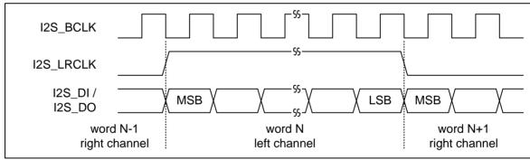
Figure 6-131 MSB Justified Data Format Timing Diagram
