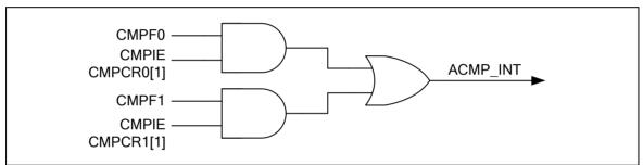
Figure 6-163 Comparator Controller Interrupt Sources
