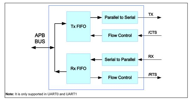
Figure 6-60 Auto Flow Control Block Diagram
