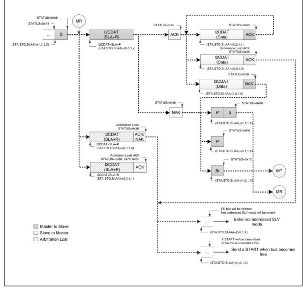
Figure 6-105 Master Receiver Mode Control Flow
