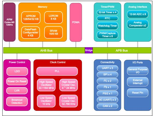
Figure 5-1 NuMicro™ NUC230 Block Diagram
