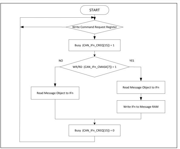
Figure 6-145 Data Transfer between IF*n* Registers and Message
