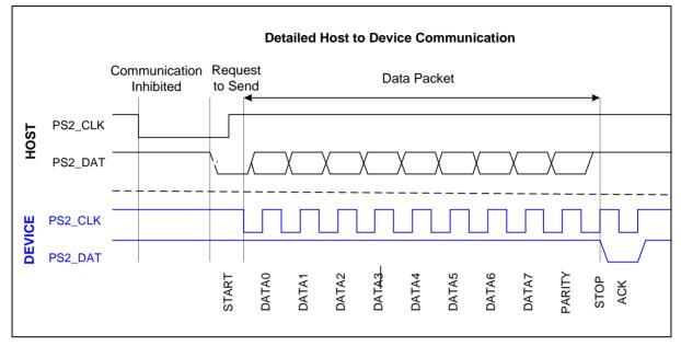
Figure 6-92 PS/2 Bit Data Format
