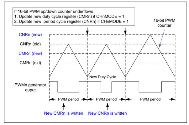
Figure 6-41 Center-aligned Type Output Waveform
