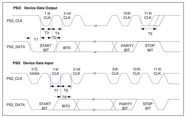
Figure 6-93 PS/2 Bus Timing
