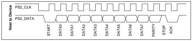
Figure 6-91 Data Format of Host-to-Device
