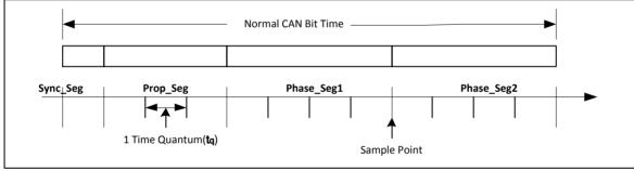
Figure 6-147 Bit Timing
