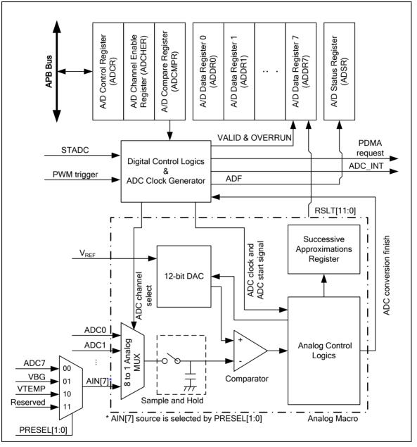
Figure 6-152 ADC Controller Block Diagram
