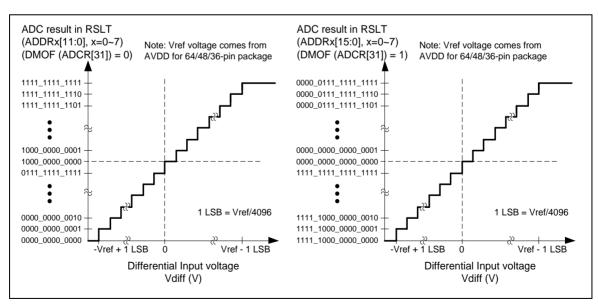
Figure 6-161 ADC Differential Input Conversion Voltage and Conversion Result Mapping
