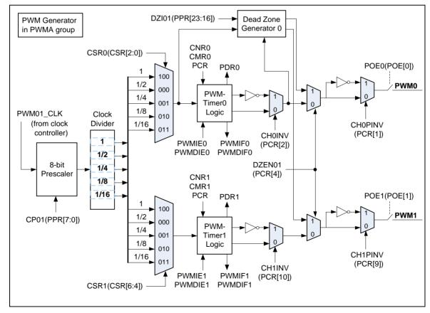
Figure 6-31 PWM Generator 0 Architecture Diagram
