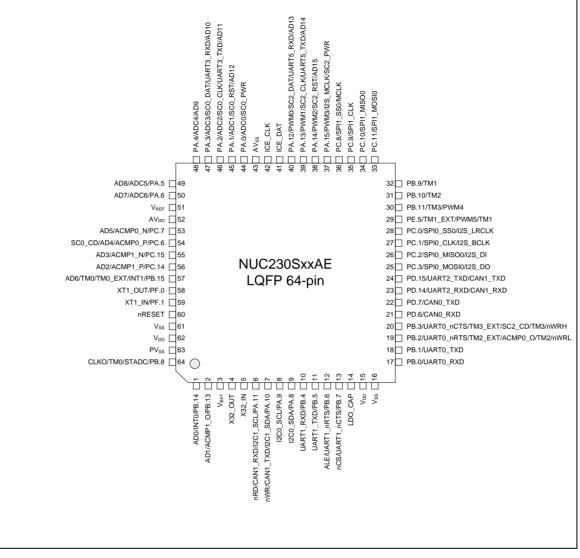
Figure 4-3 NuMicro<sup>™</sup> NUC230SxxAE LQFP 64-pin Diagram
