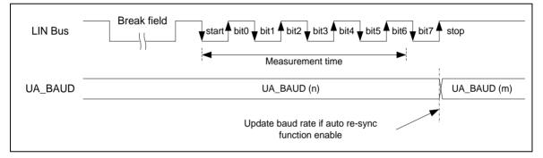
Figure 6-70 LIN Sync Field Measurement
