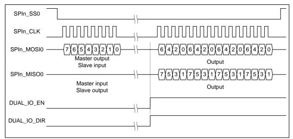
Figure 6-121 Bit Sequence of Dual Output Mode
