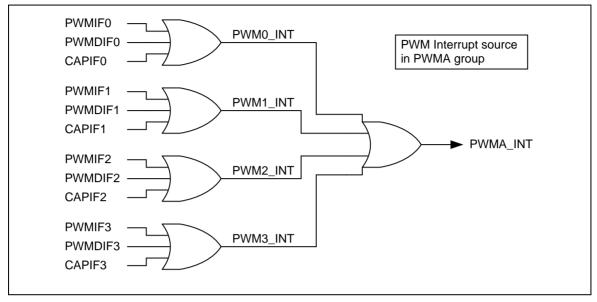
Figure 6-48 PWM Group A PWM-Timer Interrupt Architecture Diagram
