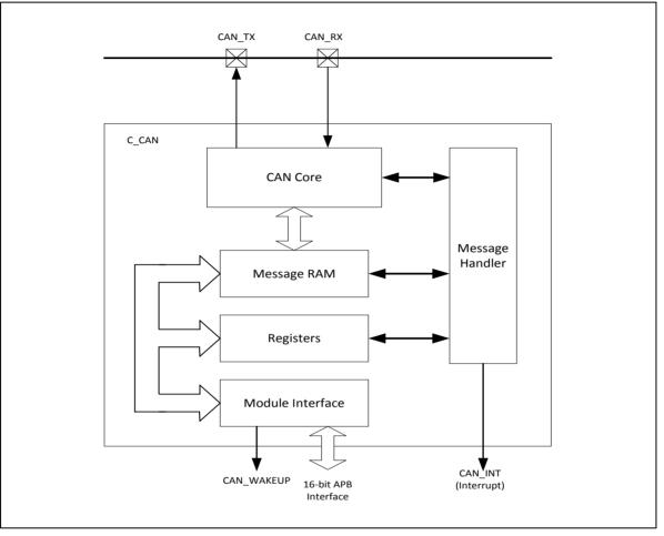
Figure 6-141 CAN Peripheral Block Diagram
