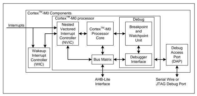
Figure 6-1 Functional Controller Diagram
