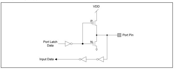
Figure 6-22 Push-Pull Output
