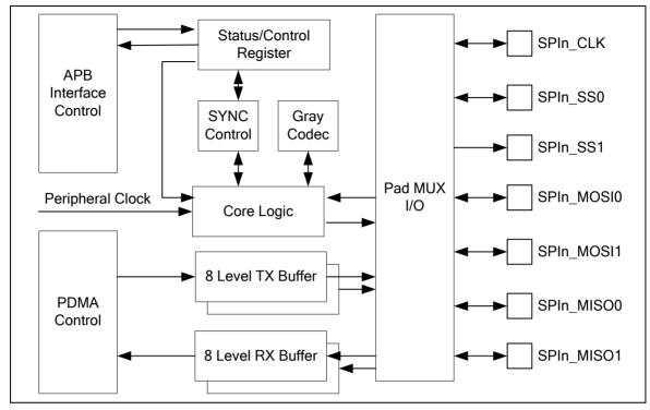
Figure 6-113 SPI Block Diagram
