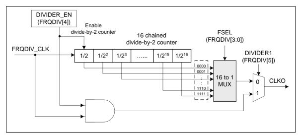
Figure 6-9 Frequency Divider Block Diagram
