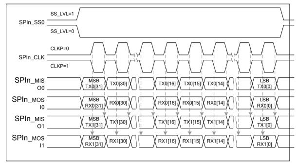
Figure 6-120 2-bit Transfer Mode (Slave Mode)
