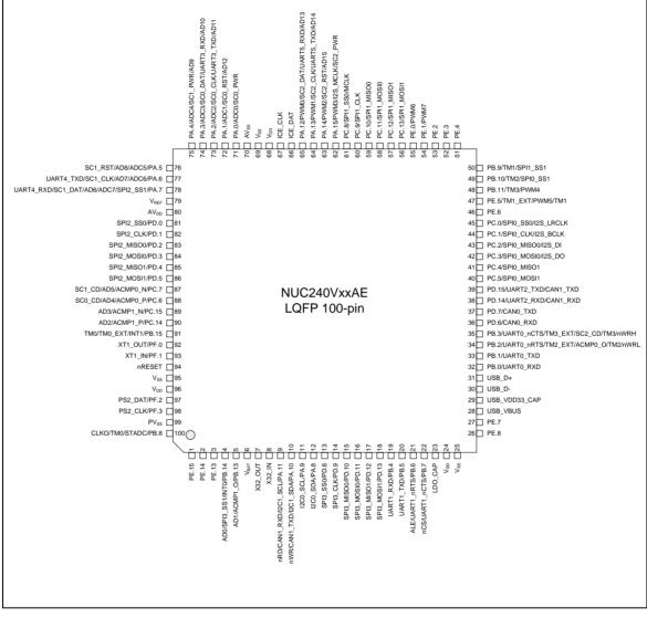
Figure 4-5 NuMicro™ NUC240VxxAE LQFP 100-pin Diagram
