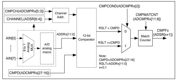
Figure 6-158 A/D Conversion Result Monitor Logics Diagram
