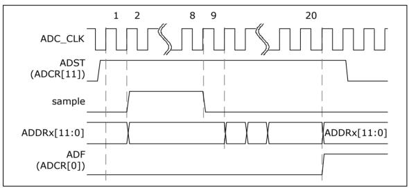
Figure 6-154 Single Mode Conversion Timing Diagram
