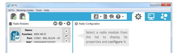
3. Click the Radio Module to read the current configuration. The radio configuration appears on the right side of the screen. All available parameters for configuration of the module are listed in this section. Each individual parameter for configuration of the module is listed in this section and can be refreshed and written to the module using this tool.
