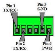
The following figure shows the pins used on the RS-485 (2 wire) Phoenix 6-pin connector:
