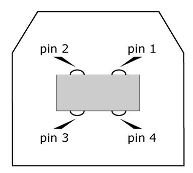
The following figure shows type B USB connector pin assignments and implementation:
