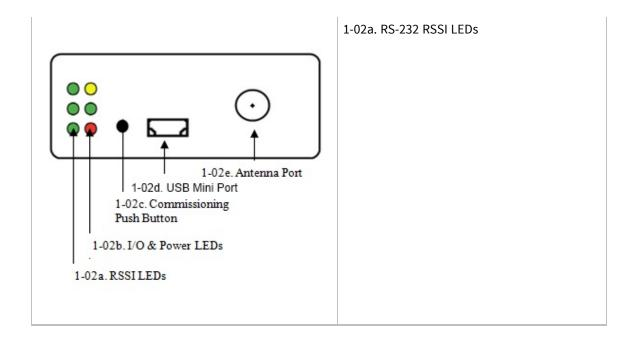
RSSI LEDs indicate the amount of fade margin present in an active wireless link. Fade margin is defined as the difference between the incoming signal strength and the modem's receiver sensitivity.
