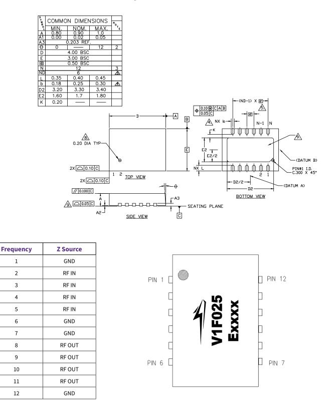
Note: Leadframe finish for 3x4 DFN package is Nickel/Palladium/Gold. Gold is the outer layer
