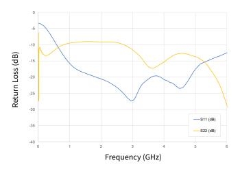
Figure 2. Input & Output Return Losses vs Frequency  $V_{DD} = 50 \text{ V}$ ,  $I_{DO} = 500 \text{ mA}$
