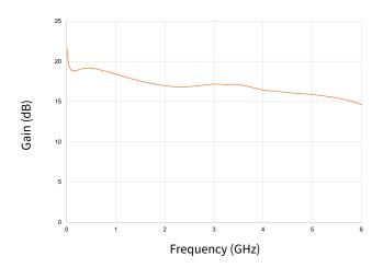
Figure 1. Small Signal Gain vs Frequency  $V_{DD} = 50 \text{ V}, I_{DO} = 500 \text{ mA}$
