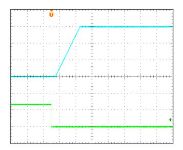
Figure 4: Remote On/Off(negative logic) at full load
