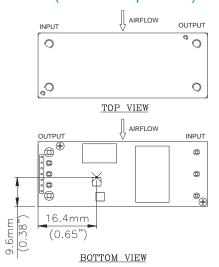
**Figure 17:** Hot spot 1 temperature measurement location The allowed maximum hot spot 1 temperature is defined at 124  $\mathcal{C}$ .
