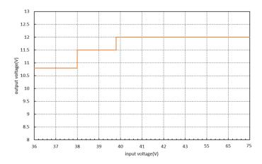
Figure 3: Output voltage vs. input voltage for open load at 25  $\!\!\!\!\!\!\!^{\circ}\!\!\!\!\!\!\!^{\circ}$  .
