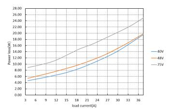
Figure 1: Efficiency vs. load current for 40V, 48V, and 75V input voltage and 12V output voltage at 25  $^{\circ}$ C.
