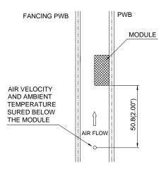
Note: Wind Tunnel Test Setup Figure Dimensions are in millimeters and (Ir
