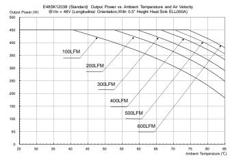
Figure 22: Output Power vs. Ambient Temperature and Air Velocity @Vin = 48V ((Longitudinal Orientation, Airflow from Input to Output, With 0.5" Height Heat Sink ELL050A)
