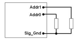
Corresponded to each octal digit, the requested resistor values are shown in below, and +/-1% resistors accuracy can be accepted. If there are any resistances exceeding the requested range, address 126 will be return. 0-12 and 40, 44, 45, 55 and 63 in decimal address can't be used, since they are reserved according to the SMBus specifications, and which will also return address 126.
