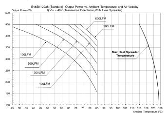
Figure 18: Output Power vs. Ambient Temperature and Air Velocity @Vin = 48V (Transverse Orientation, Airflow from Vin+ to Vin-, With Heat Spreader)
