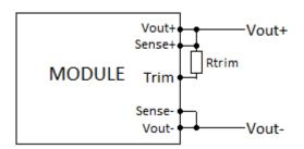
Figure 15: Circuit configuration for trim-up (increase output voltage)
