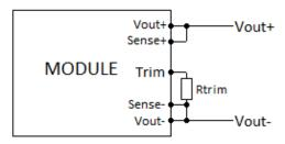
Figure 14: Circuit configuration for trim-down (decrease output voltage)
