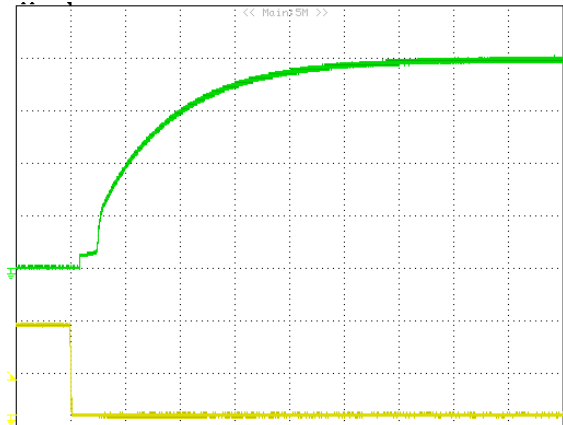
Figure 5: Turn-on transient at zero load current (10 ms/div). Vin=48V. Top Trace: Vout: 3.0V/div, Bottom Trace: ON/OFF input, 3V/div
