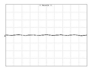
**Figure 10:** Input reflected ripple current,  $i_s$ , through a  $12\mu H$  source inductor at nominal input voltage (vin=48v) and rated load current (20 mA/div, 1us/div)
