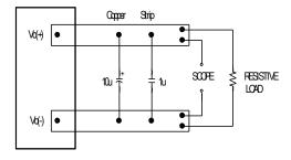
Figure 11: Output voltage noise and ripple measurement test setup
