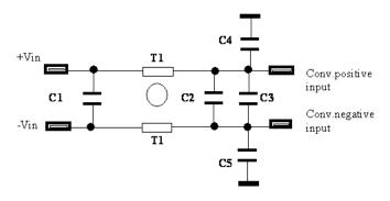
C1=3.3uF /100 V ceramic cap; C2=C3= 47 uF/100V low ESR Aluminum cap; C4=C5=1nF/250Volt ceramic cap; T1=3 mH
