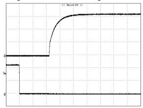
Figure 4: Turn-on transient at full rated load current (resistive load) (10 ms/div). Vin=48V. Top Trace: Vout, 1.0V/div; Bottom Trace: ON/OFF input, 2V/div
