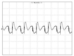
Figure 12: Output voltage ripple at nominal input voltage (vin=48v) and rated load current (Io=15A) (50 mV/div, 1us/div). Load capacitance: 1μF ceramic capacitor and 100μF tantalum capacitor. Bandwidth: 20 MHz. Scope measurements should be made using a BNC cable (length shorter than 20 inches). Position the load between 51 mm to 76 mm (2 inches to 3 inches) from the module
