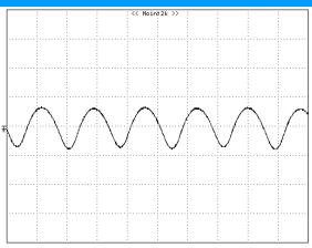
Figure 9: Input Terminal Ripple Current, ic, at full rated output current and nominal input voltage (Vin=48v) with 12μH source impedance and 33μF electrolytic capacitor (200 mA/div, 1us/div)
