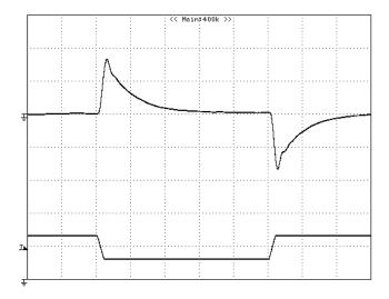
Figure 7: Output voltage response to step-change in load current (50%-25%-50% of Io, max; di/dt = 0.1A/μs; Vin is 48v). Load cap: 10μF tantalum capacitor and 1μF ceramic capacitor. Top Trace: Vout (50mV/div, 200us/div), Bottom Trace: lout (5A/div). Scope measurement should be made using a BNC cable (length shorter than 20 inches). Position the load between 51 mm to 76 mm (2 inches to 3 inches) from the module.
