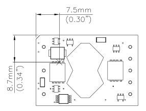
**Figure 19:** Temperature measurement location  $^*$  The allowed maximum hot spot temperature is defined at 118  $\mathcal{C}$ .
