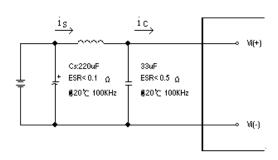
**Figure 8:** Test set-up diagram showing measurement points for Input Terminal Ripple Current and Input Reflected Ripple Current.
