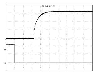
Figure 5: Turn-on transient at zero load current (10 ms/div). Vin=48V. Top Trace: Vout: 1.0V/div, Bottom Trace: ON/OFF input, 2V/div
