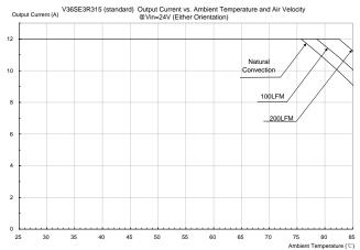
Figure 20: Output current vs. ambient temperature and air velocity @ V<sub>in</sub>=24V (Either Orientation)
