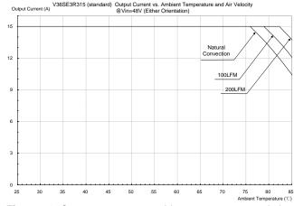
**Figure 21:** Output current vs. ambient temperature and air velocity @ V<sub>in</sub>=48V (Either Orientation)
