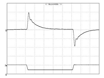
Figure 6: Output voltage response to step-change in load current (50%-25%-50% of lo, max; di/dt = 0.1A/µs; Vin is 24v). Load cap: 10µF tantalum capacitor and 1µF ceramic capacitor. Top Trace: Vout (50mV/div, 200us/div), Bottom Trace: lout (5A/div). Scope measurement should be made using a BNC cable (length shorter than 20 inches). Position the load between 51 mm to 76 mm (2 inches to 3 inches) from the module.
