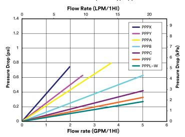
Graph 1: Polypropylene Filter Flow Comparison
