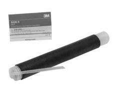
They are factory expanded and assembled onto a core which is removed after the tube has been positioned for installation over an inline connection or harness section. The tube shrinks, forming a dynamic, environmental seal which resists prolonged aging and exposure. It installs quickly with little training and no tools or heat source.
