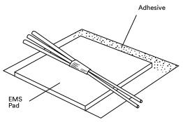
NOTE: Do not hold wires while compressing pad. Hydraulic pressure from compressed adhesive will flair the wires automatically causing the adhesive to flow between and seal the wires. Pressed pads may be reshaped to make the covered junction more compact.
