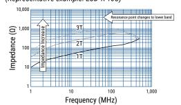
Figure 3 - Effective band range of Nanocrystal core material.
