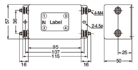
Recommended torque (N-m) maximum • Line terminal (M4: 0.78)
