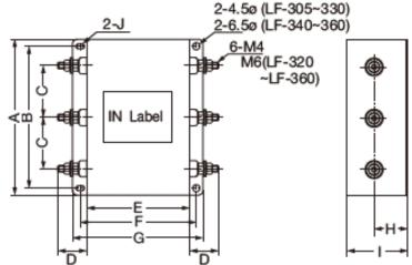
Recommended torque (N-m) maximum • Line terminal (M6: 1.18)
