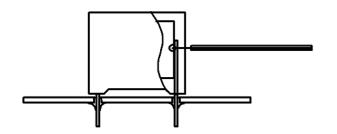
Temperature monitored inside the capacitor.
