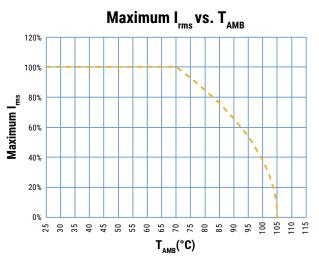
$T_{AMB}$  is the maximum ambient temperature surrounding the capacitor or hottest contact point (e.g. tracks), whichever is higher, in the worst operation conditions in °C.
