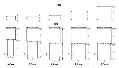
$\textit{F case size is the same as D, but with 0.200" (5.0 \, mm) lead spacing. Specify T340F \textit{ when ordering this spacing.} \\$
